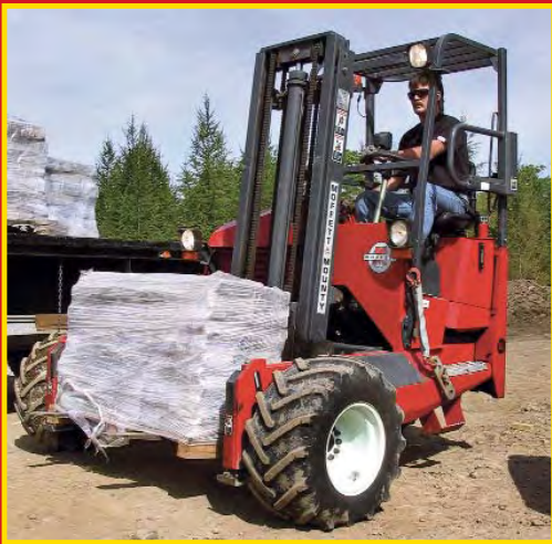
Transporting skids on site with the all-wheel drive Moffett Mounty forklift.
