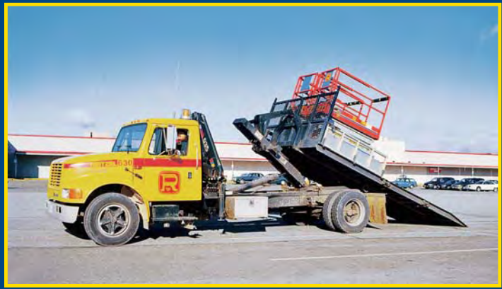
Moving rental equipment with a versatile Multilift Hooklift demountable body system and HIAB truck crane package.
