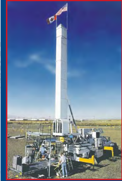
Spar Aerospace and Atlas Polar worked jointly to develop and install special truck and trailer mounted frameworks for four Canadarm type robotic units designed for hazardous waste inspection and clean-up.
