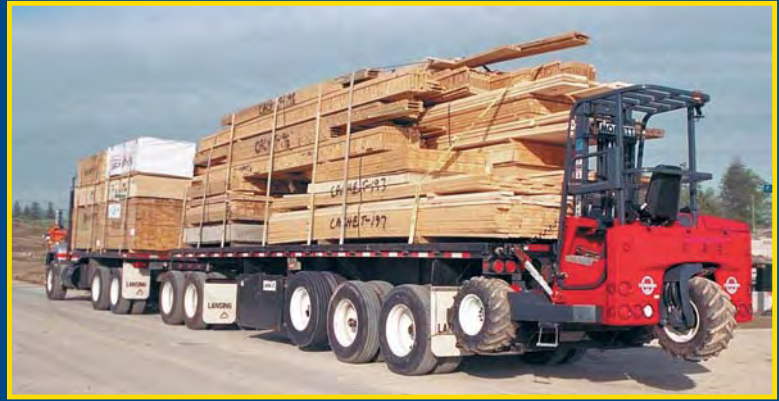
Deliver products to DIY's and contractors the fast and easy way with a Moffett Mounty forklift stored at the rear of a truck or trailer.
