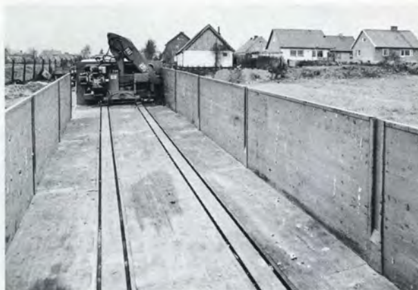
The firm's latest purchase is equipped with a HIAB 174 mounted on a roller track. With this arrangement the crane can not only reach all over the deck but can also be rolled across onto the tractor truck if need be.
