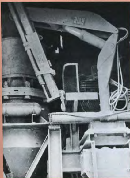
In the sorting department is a finishing crusher, and this machine too has a crane for servicing work. In these narrow confines the choice fell on a HIAB 174.
