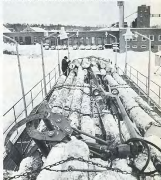
During travelling the loader jib is placed above the timber pile in the middle.
