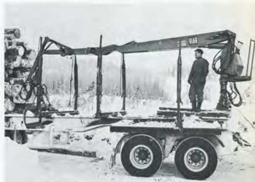
Here is the crane advanced to its foremost position for loading up the last lot of timber, the pile in the middle. Notice the additional articulation joint with which the jib of the crane is equipped. It functions automatically in connection with the operation of the extension, giving increased reach and making it easier to work close in to the loader column.
