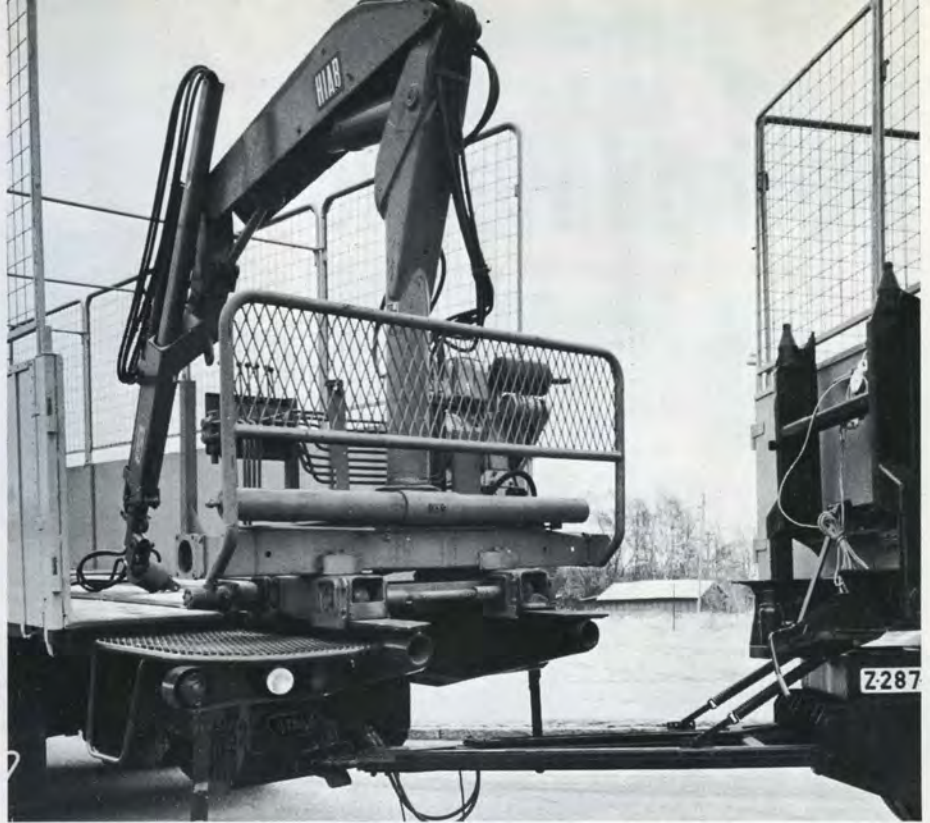
A pair of stout rails can be swung down to form a continuation of the frame side-members so that the crane can be run across between tractor truck and trailer.
