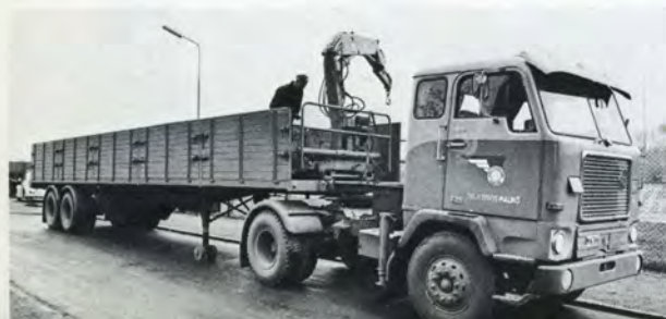
The firm's latest purchase is equipped with a HIAB 174 mounted on a roller track. With this arrangement the crane can not only reach all over the deck but can also be rolled across onto the tractor truck if need be.
