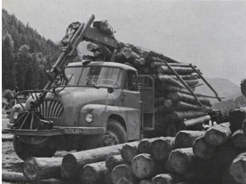
The roads through the forests of this near-Alpine terrain pose big problems for heavy rigs. This six-wheeler is operated without a trailer, and both axes of the bogie are powered. In a tight spot the drive can be clutched to the front wheels as well.
