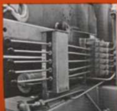
Valve unit with replaceable valve sections; can easily be augmented with additional valve functions.
