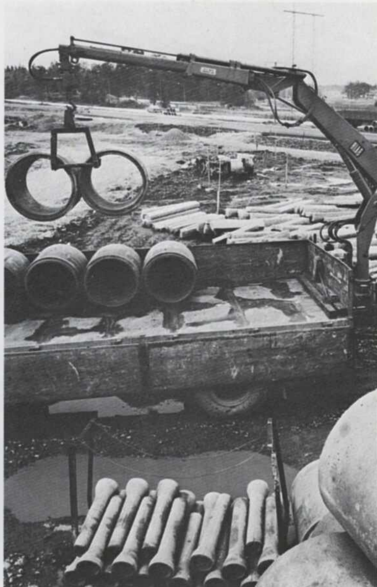
The hydraulic extension of the 174 makes it easy to stack up high piles, and the rotator permits precise positioning, which prevents impact damage to pipes.
