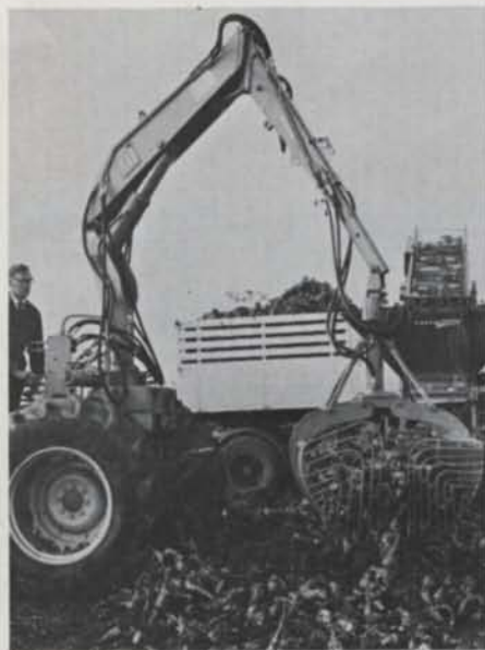
Beet loading being demonstrated at an agricultural show. The equipment seen behind the basket-equipped Speedloader removes some of the soil and tares from the beets before they go aboard the truck. The outfit on the right is equipped with a HIAB 173 Speedloader and is used as an all-round crane.
