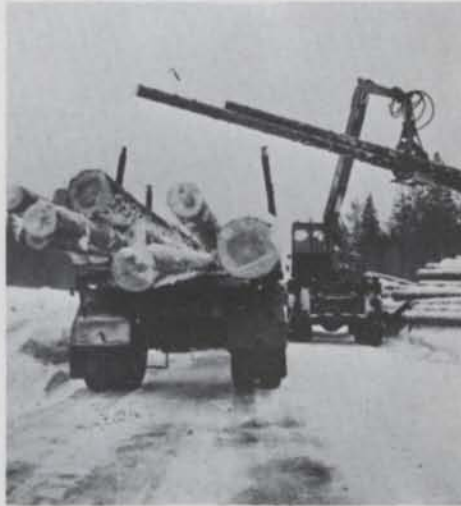
Here's a sensible way to use a transport rig. It shuttles between two towns way up north in Sweden, about 180 miles apart. On the outward trip it carries concrete beams to building sites, and on the way back it takes steel sheet from the North Bothnian Steelworks. Loading and unloading are looked after by a HIAB 174 Speedloader side-mounted half way along the deck so as to be able to lift the heavy freight at its centre of gravity. The picture on the left shows how the 174 tucks snugly away behind the flaps.
