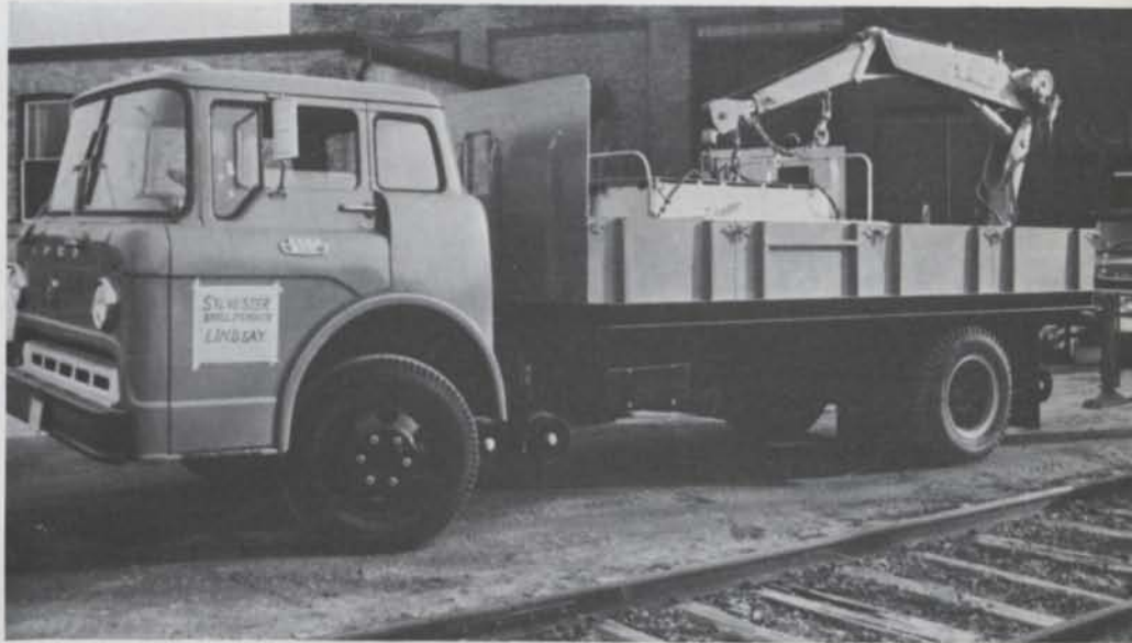
The picture above shows the "rail/road truck" standing alongside the track with its dolly wheels and support legs retracted.
