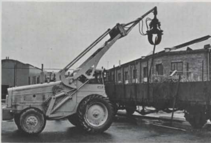
The polygrip bucket begins by lifting the tarpaulin off the car and then picks out the stanchions one by one.
