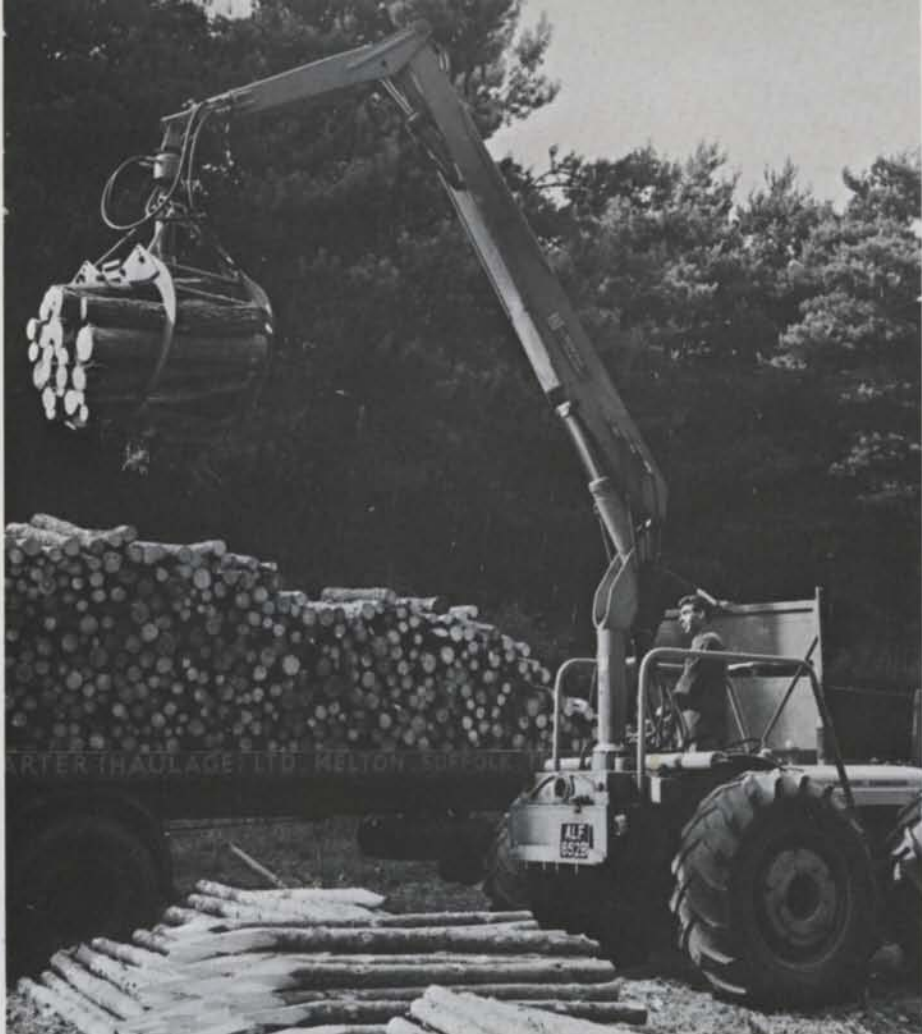
British pulpwood is a good deal shorter than Swedish foresters are accustomed to. The grapple load is therefore less, so that the tractor carrying this Forest Speedloader can dispense with support legs.
