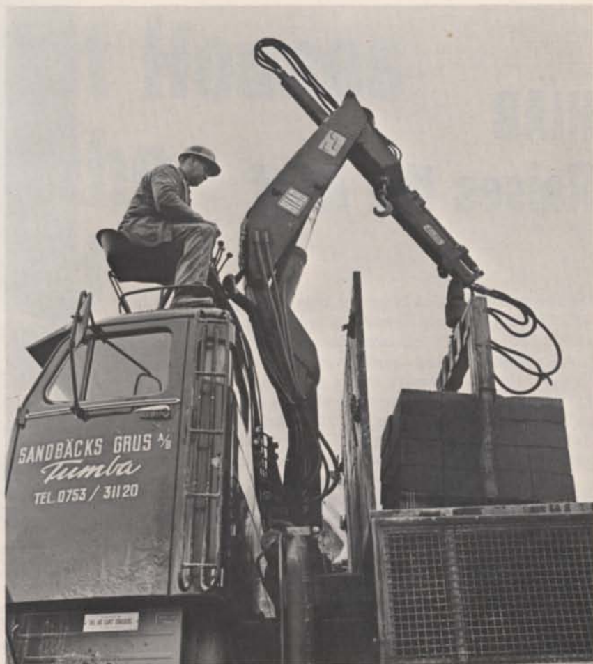
These cement blocks are being handled by a HIAB 174 Speedloader equipped with a special clamp. The driver in the upper picture operates from a control seat sited on the cab roof, giving him an excellent view of the job and making it easier to deposit the pallets just where he wants them. This arrangement also retains the short distance between the front wall of the deck and the back of the cab. The seat is collapsible so as not to make the outfit unnecessarily high. In the lower picture the driver is operating the rear-mounted loader from a special platform. And here we can see just how the blocks are put down right where they are to be used, so that the building workers do not have to bother with unloading at all.
