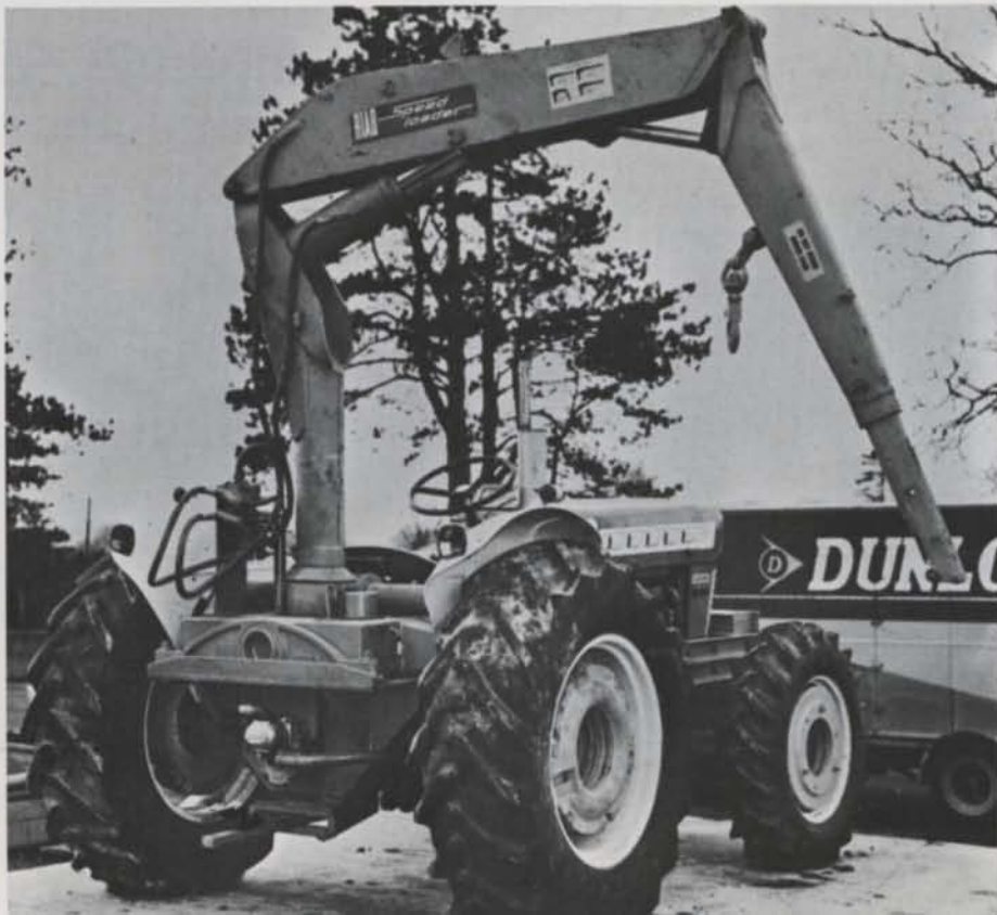
Beet loading being demonstrated at an agricultural show. The equipment seen behind the basket-equipped Speedloader removes some of the soil and tares from the beets before they go aboard the truck. The outfit on the right is equipped with a HIAB 173 Speedloader and is used as an all-round crane.
