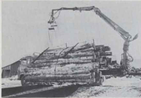
Torgren's Sawmill at Kvarnåsen in Northern Sweden collects its timber supplies with its own trucks, which are naturally equipped with HIAB 177 Speedloaders. The lengthy reach of these cranes is essential for picking up timber piles which are often small and are not always as close to the road as they might be. The load is discharged by the bundle at the sawmill.
