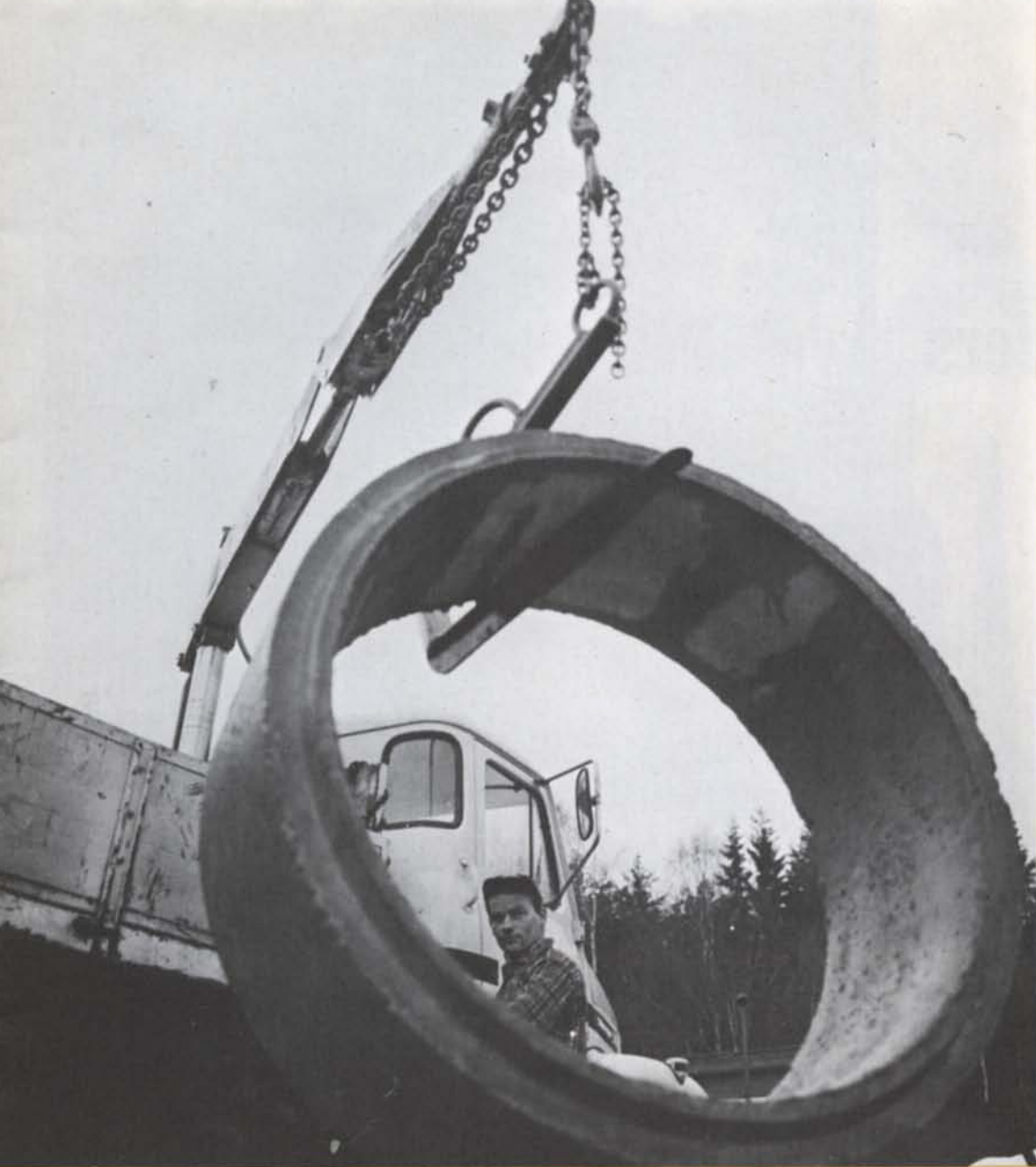
Dahiströms Betonggjuteri, a precast-concrete firm in a small Swedish town, bought a new delivery truck a year ago. It is mostly used for short hauls of around 25-30 miles. With a HIAB 293 the driver can handle even the largest concrete rings, and the truck has a larger payload than it would have if it carried a bigger crane.
