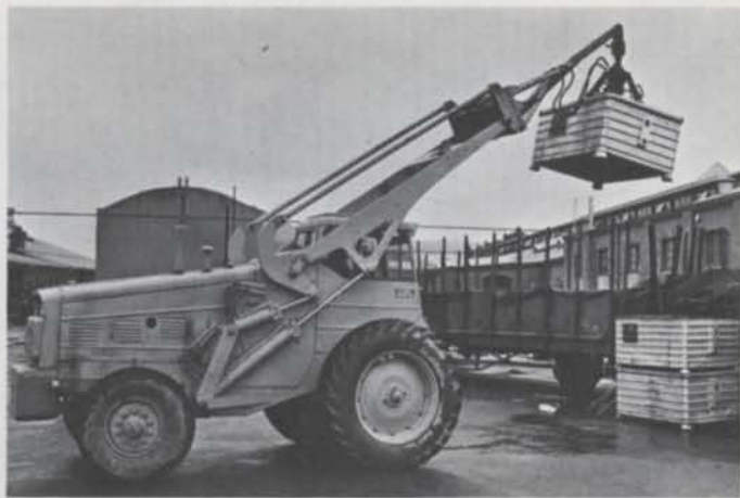
Once the flaps have been lowered, the containers into which the scrap is to be discharged are lifted into position by the bucket, the claws of which are expanded against the insides of the containers.
