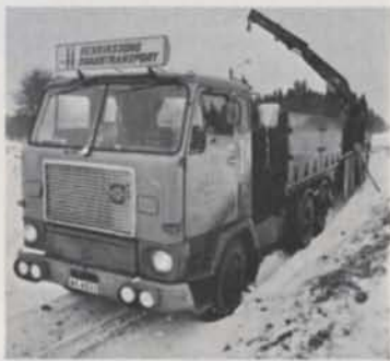
Here's a sensible way to use a transport rig. It shuttles between two towns way up north in Sweden, about 180 miles apart. On the outward trip it carries concrete beams to building sites, and on the way back it takes steel sheet from the North Bothnian Steelworks. Loading and unloading are looked after by a HIAB 174 Speedloader side-mounted half way along the deck so as to be able to lift the heavy freight at its centre of gravity. The picture on the left shows how the 174 tucks snugly away behind the flaps.
