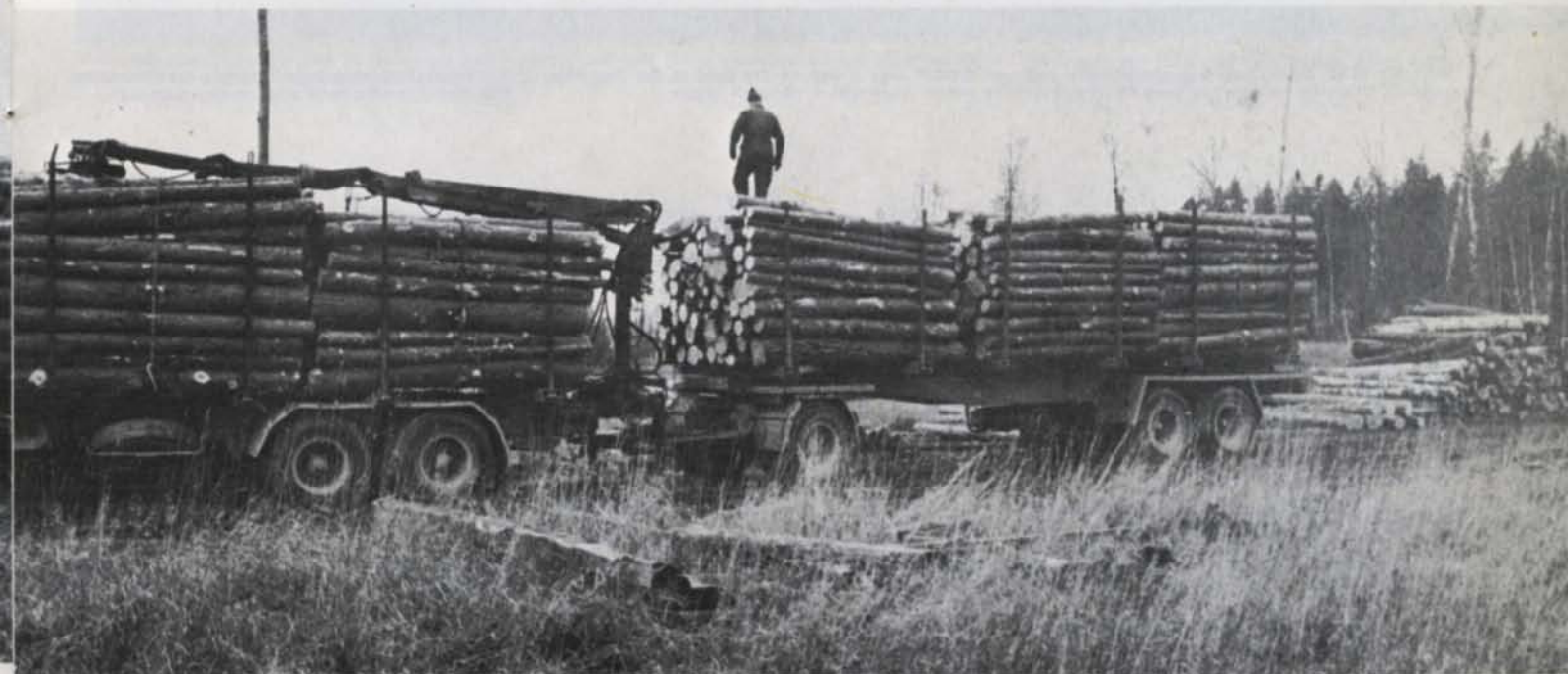
On the short timber hauls the loader rides along all the time, with the jib laid out along the top of the load like this.
