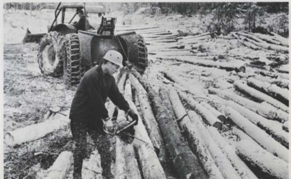
Bucking, along with any remaining trimming, is done quickly and efficiently at the landing.
