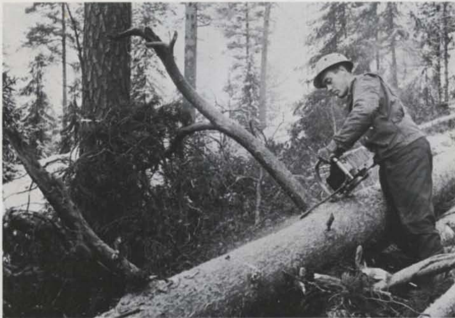
The lumberjack fells the tree in the usual way but trims off only those branches he can conveniently reach. Those on the underside he leaves untouched.
