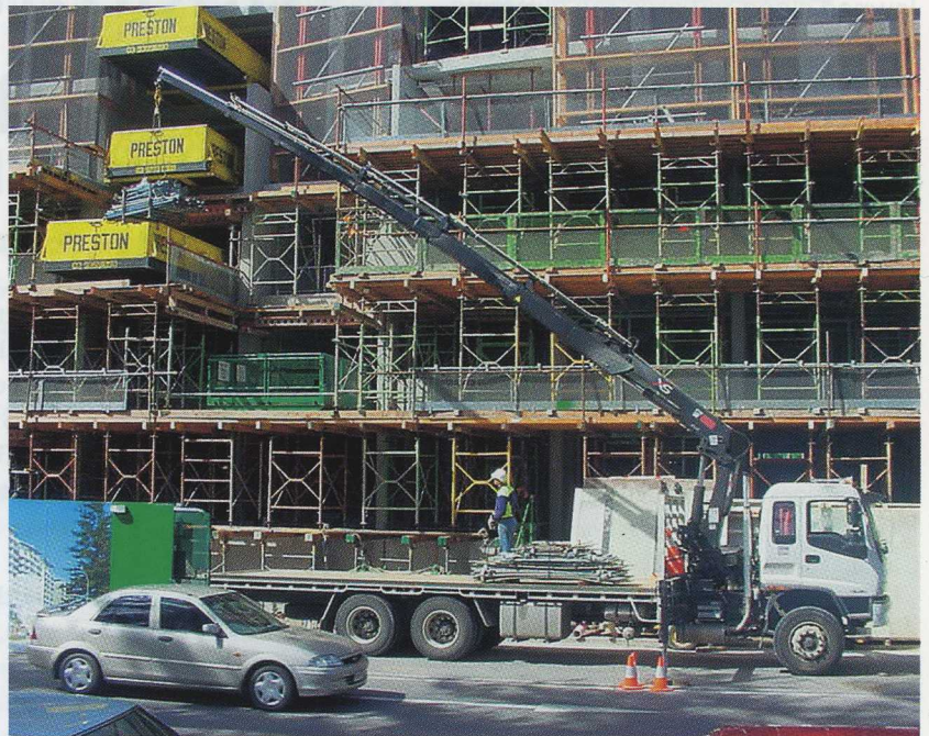
Sani Strehovski's XS 166 E-5 HiPro is the perfect tool for the distribution and erection of scaffolding.
