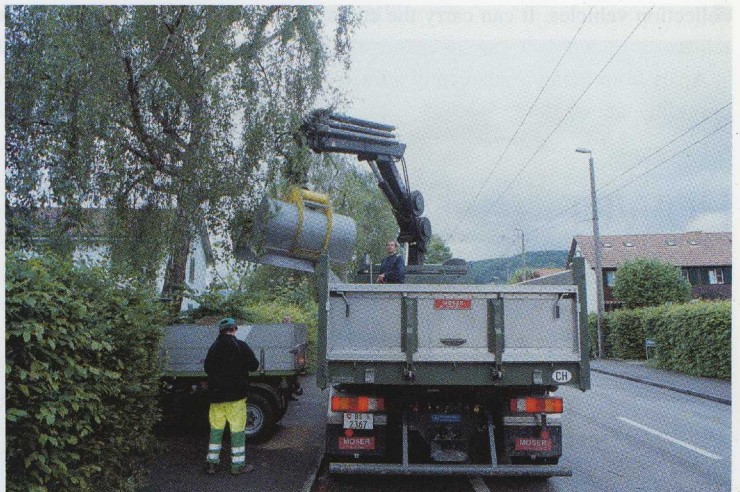
There's little space and it's fiddly, but from his platform Pierre Stutz has a clear view of the work area and can manoeuvre his XS 166 HiPro safely – and elegantly.
