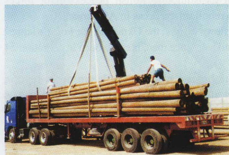
Using a HIAB 500 made light work of handling 30,000 telephone poles at the port of Callao in Peru.
