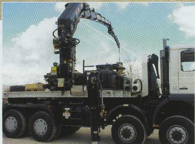
An all-round solution. With its Multilift, ART-TOIT can lift their HIAB 550-6 on-and-off according to need.
