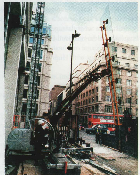
RALF is a unique machine based on a HIAB 026 T. It was designed by GGR Glass Services Ltd, of London and Rochdale, to handle window panes with dimensions of up to 7.2 x 1.6 metres and weighing up to 560 kilograms.
