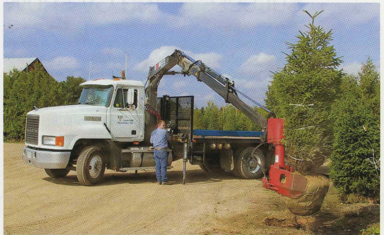
A special grab fitted to a HIAB 081 makes light work of loading fir trees for delivery. The drivers had a choice of cranes for jobs and it fell on – Hiab.
