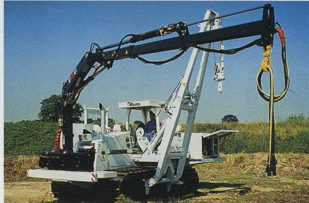
The Liebherr RL 22 B Litronic – an impressive machine, specially designed for pipeline welding work. The standard equipment includes a HIAB 071 AW, which can handle 2 tons at 3.6 metres or 1 ton at 6.9 metres.
