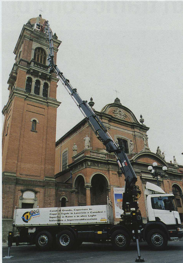
The Georgi brothers were looking for a reliable all-in-one solution and found it in the form of a HIAB 550-6 with Jib, winch, personnel basket and radio control.
