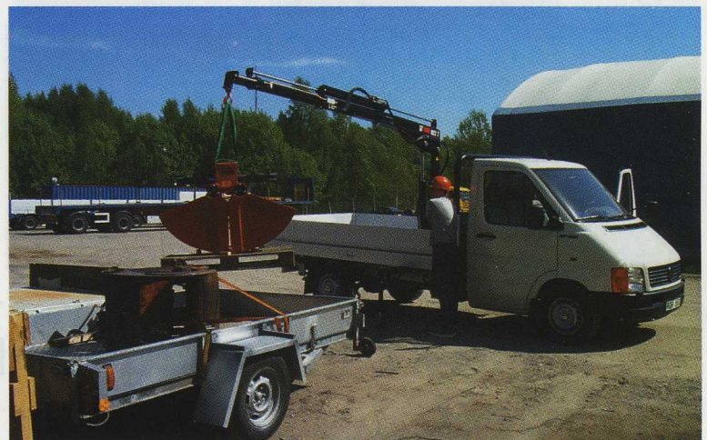
A light construction with a long outreach characterise the HIAB 022 T.
