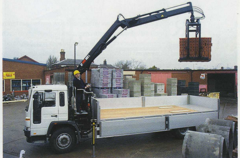
The 085 L has an extra long inner boom, which provides unbeatable power right when you need it, for example when delivering building materials.
