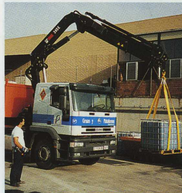
With a HIAB 245 E – mounted on a three-axle IVECO EuroTech Cursor – operator Jesus Rodriguez Magallón can handle a whole range of tricky jobs. This is one of the easier ones...
