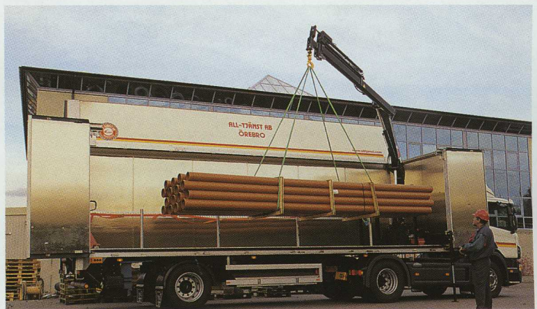
On the road, it looks like any other large delivery van. However, as a tractor and trailer combination it can manoeuvre into the tightest of spaces. The sidewalls and roof open up and on the load platform inside is a HIAB 060, ready to get to grips with some heavy shifting work.
