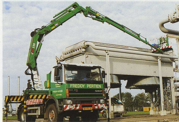
Freddy Pertien's HIAB 330 with a jib and personnel basket being used here in maintenance work alongside a heat exchanger.
