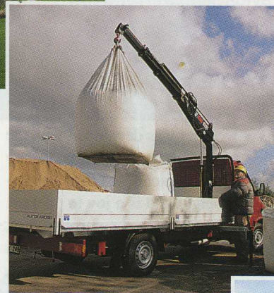
The HIAB 026-T, the strongest of the "little 'uns". Its weight, depending on the version, varies between 250-295 kg, but it can lift 1.9 tonnes.
