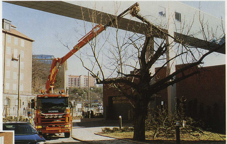
Stisse's orange Scania with its specially equipped HIAB 135-4 fells trees one bit at a time. "It's fast and it works well," Stisse tells us.
