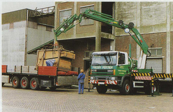
Freddy Pertien's HIAB 330 with a jib and personnel basket being used here in maintenance work alongside a heat exchanger.
