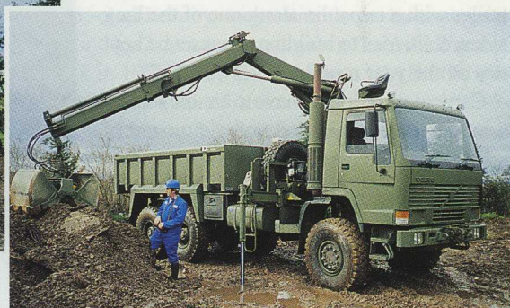
The crane can be operated from the top seat or ... ...from a more mobile position on the ground.
