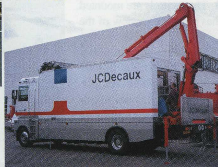
This truck regularly turns up at fairs and exhibitions around Europe. With the roof of the truck open, The HIAB 195-2, resplendoured in "JCDecaux Red", does all the lifting, while the driver keeps an eye on things from the platform at the rear.
