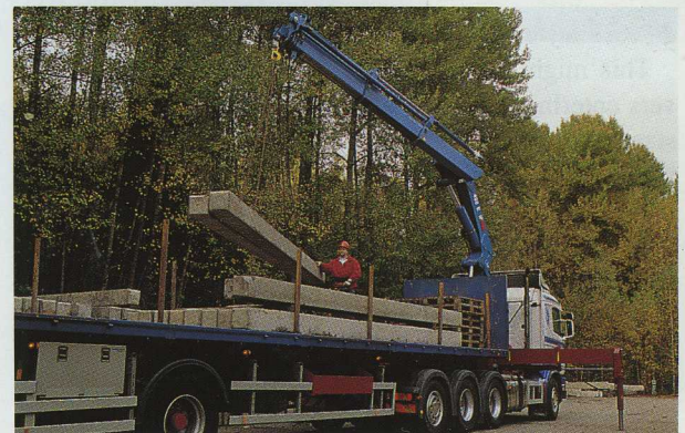
With eight hydraulic extensions the HIAB 400 E reaches 21.4 metres where it has a lifting capacity of 890 kg.
