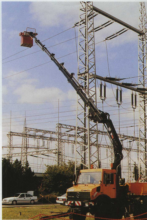
A Unimog U2450, with a winch and HIAB 245-7, fitted with a personnel basket has proved to be the ideal solution for service and maintenance work at Preussen Elektra.
