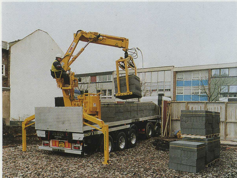
With the trailer closed up, Mick Thompson can manoeuvre into the most restricted spaces to unload.
