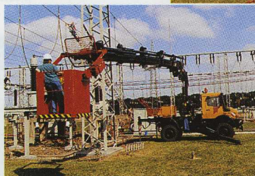
A Unimog U2450, with a winch and HIAB 245-7, fitted with a personnel basket has proved to be the ideal solution for service and maintenance work at Preussen Elektra.
