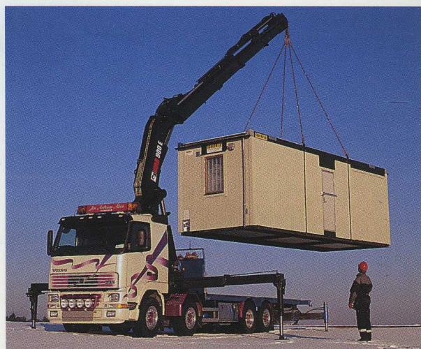
The HIAB 900 E-6 enables Jim Aaltonen to work in an entirely new way. "...particularly when handling goods beyond the immediate area of the truck." he says, "I can lift 4 tonnes to an outreach of 16.5 metres now."
