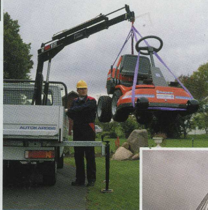
The HIAB 013-T enables drivers themselves to handle most loads normally carried on light commercial vehicles.
