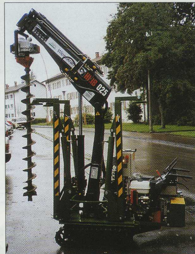
The EuroMulti crane can be equipped with tools such as augers and buckets.
