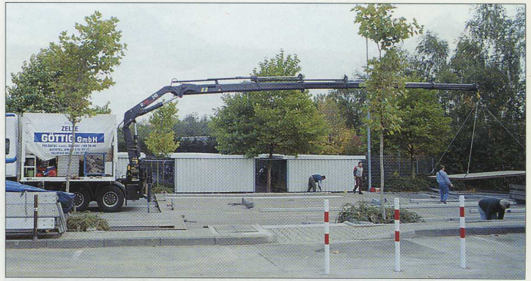
The handling of large tents is much easier now with the long reach of the HIAB 245-7.
