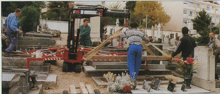
The EM crane is only 60 cm wide in transit but expands when working. So it is perfect for such places as cemeteries where access is otherwise quite difficult.
