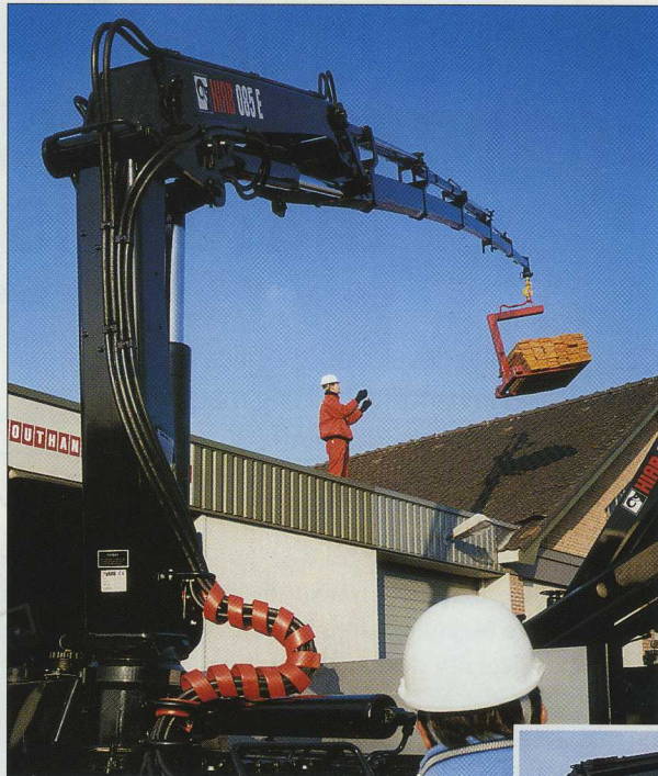
The new HIAB 085 comes in several designs including the HIAB 085 E with a double link system ...
