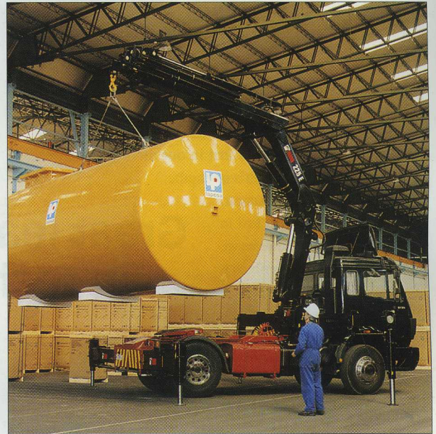
With seven hydraulic booms the reach on the HIAB 225 E and the 245 E is 19.3 metres which increases with jib and manual boom to 25.8 metres.
