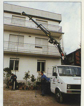
A.M.A. Ravenna's small works vehicle is used mainly for handling heavy pumps at the council's various sewage works, but is ideal for other small jobs as well.
