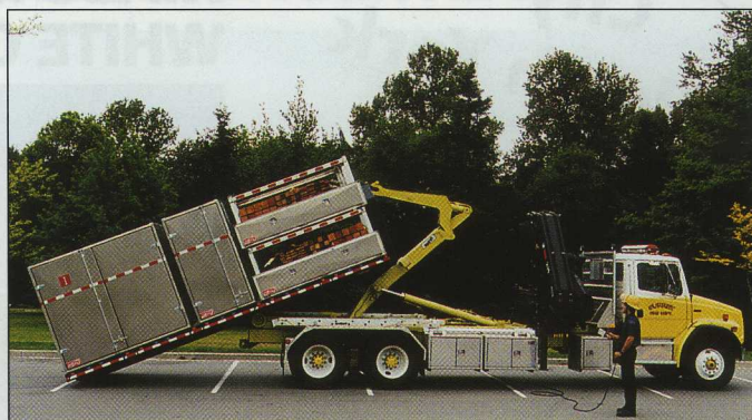
An array of different containers for different needs are loaded by one man and the HL Multilift - in two minutes!
