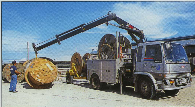
With the help of a HIAB crane, handling cable drums is very efficient.
