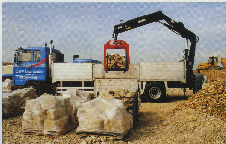
With the help of a grapple, it's easy to load pallets. With the crane the operator is able to unload without damaging lawns and plants, the customers love it!
