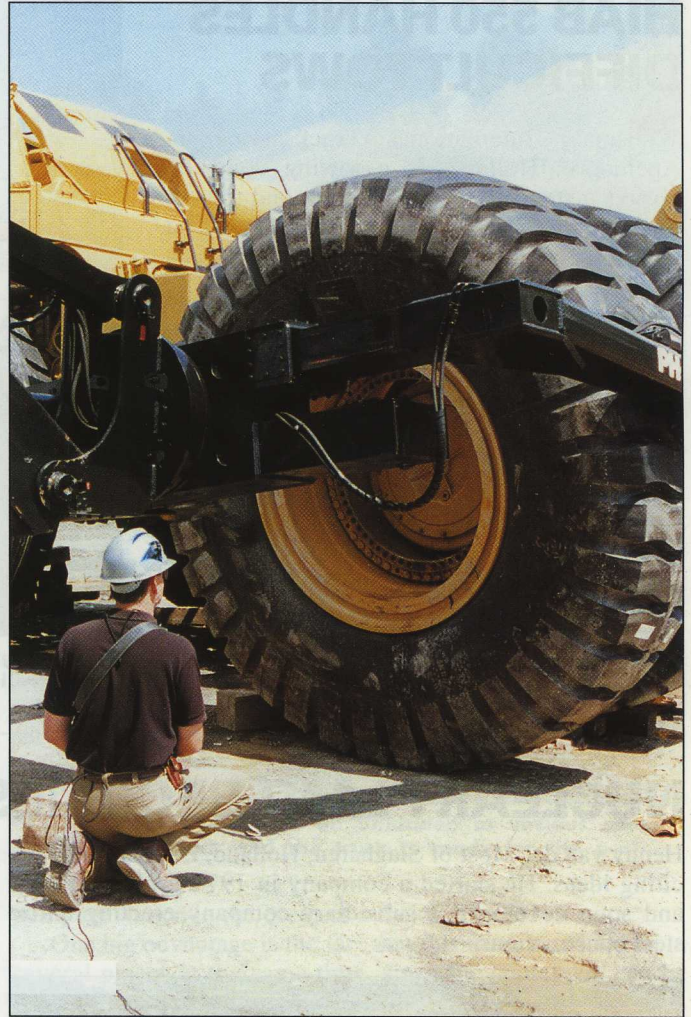
The specially designed tire grapple makes it possible to turn and wriggle this huge tire in place. Using remote control, it's easier than changing tires on your own car.
