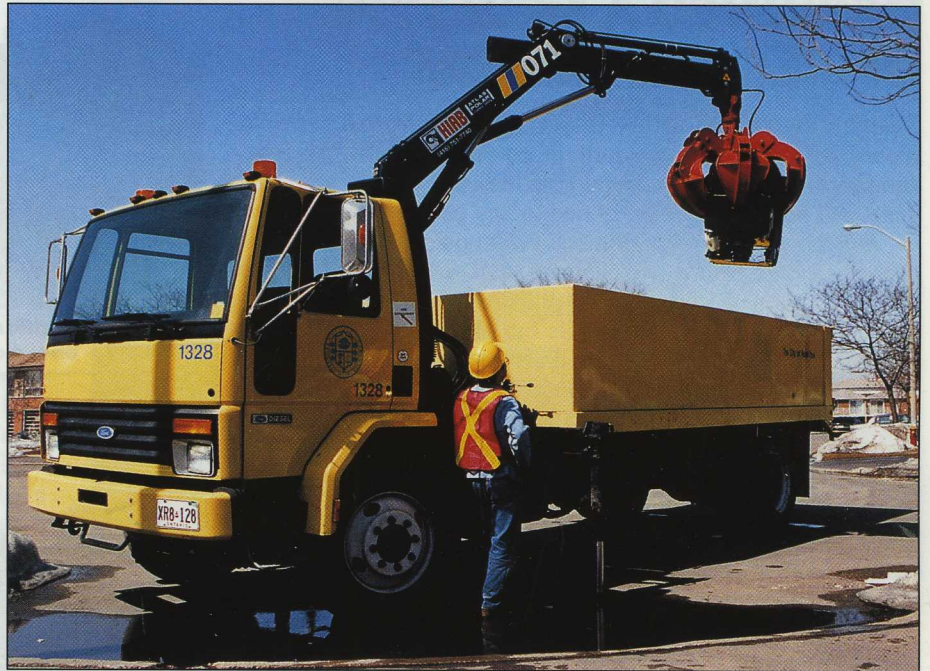
This driver, employed by the City of North York, manages singlehanded to collect rejected white goods with the help of a HIAB crane and a grapple.
