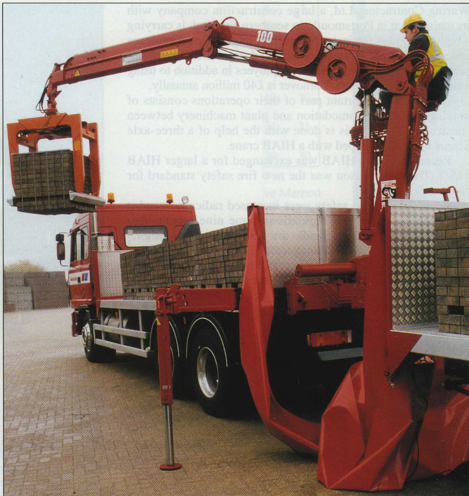
Geoff Andrew's HIAB 100 A with a top-seat, a solution he is very happy about.
