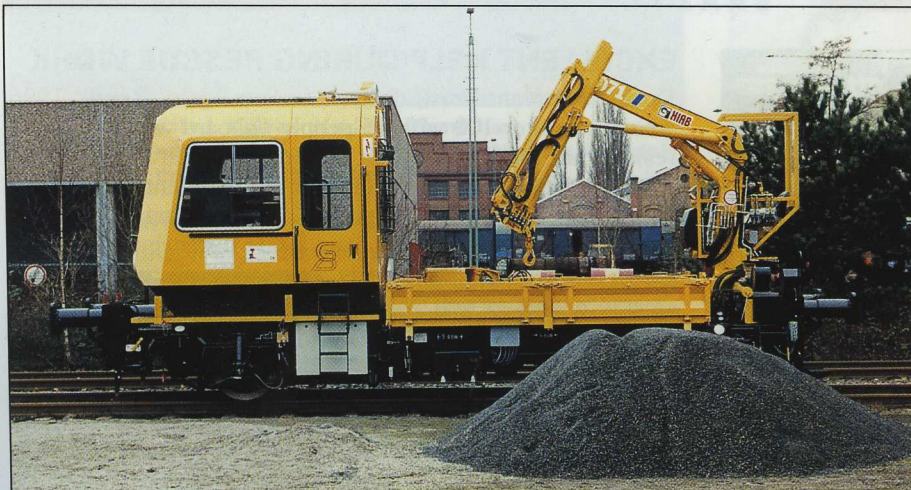
The new track construction vehicle GAF 100 R with a HIAB 071 AW and equipped with a specialized weatherproof top-seat.
