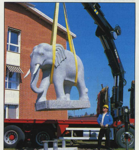
This six ton whopper was Hiab's 50th anniversary present from the Danish distributor Sawo. It was carved from granite in Thailand and was erected at the main office in Sweden with a SPACE equipped HIAB 330.
