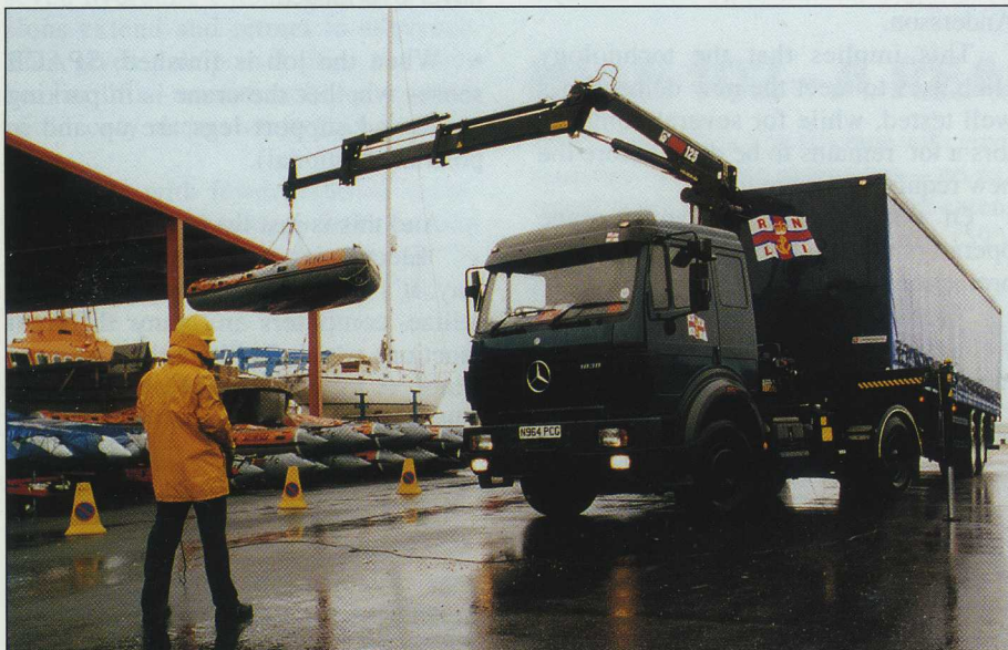
Today Tam Martin loads inflatable boats alone at the central depot in Poole with the help of his remote control HIAB 125-4.
