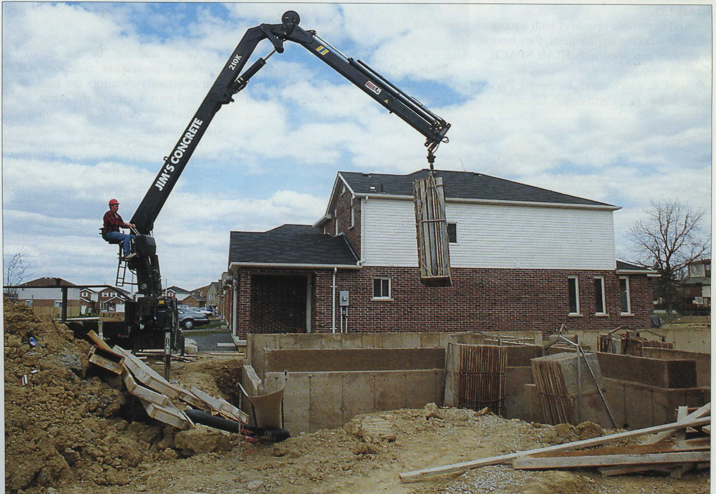
With its new balanced rack and pinion slewing system the HIAB 210 K has enough torque to rotate a full load up a four degree slope.
