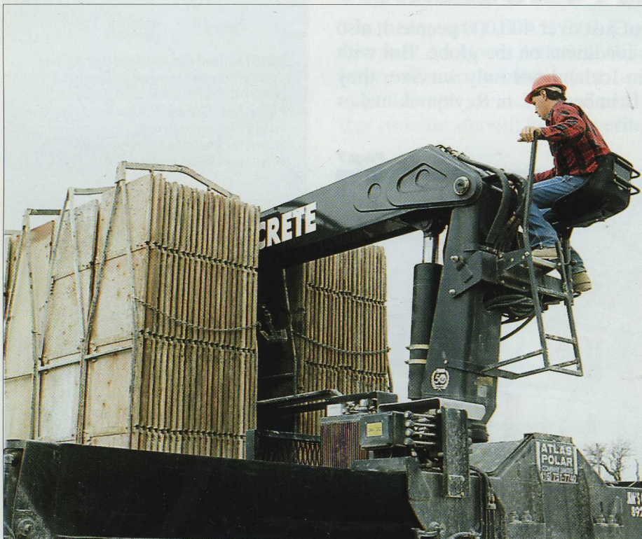
The new HIAB 210K can be easily stowed between the forming cages. Both these cranes have standard North American JIC fittings on all hoses and pipes.
