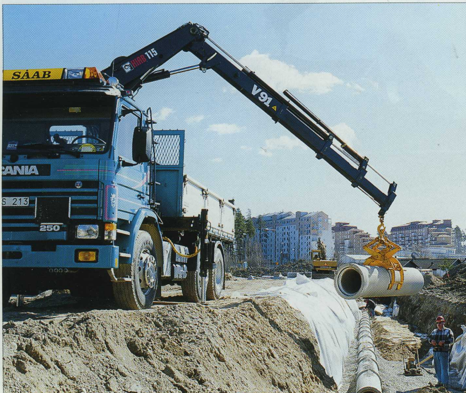
With three hydraulic extensions, the HIAB 115 has a reach of almost 9.5 metres.
