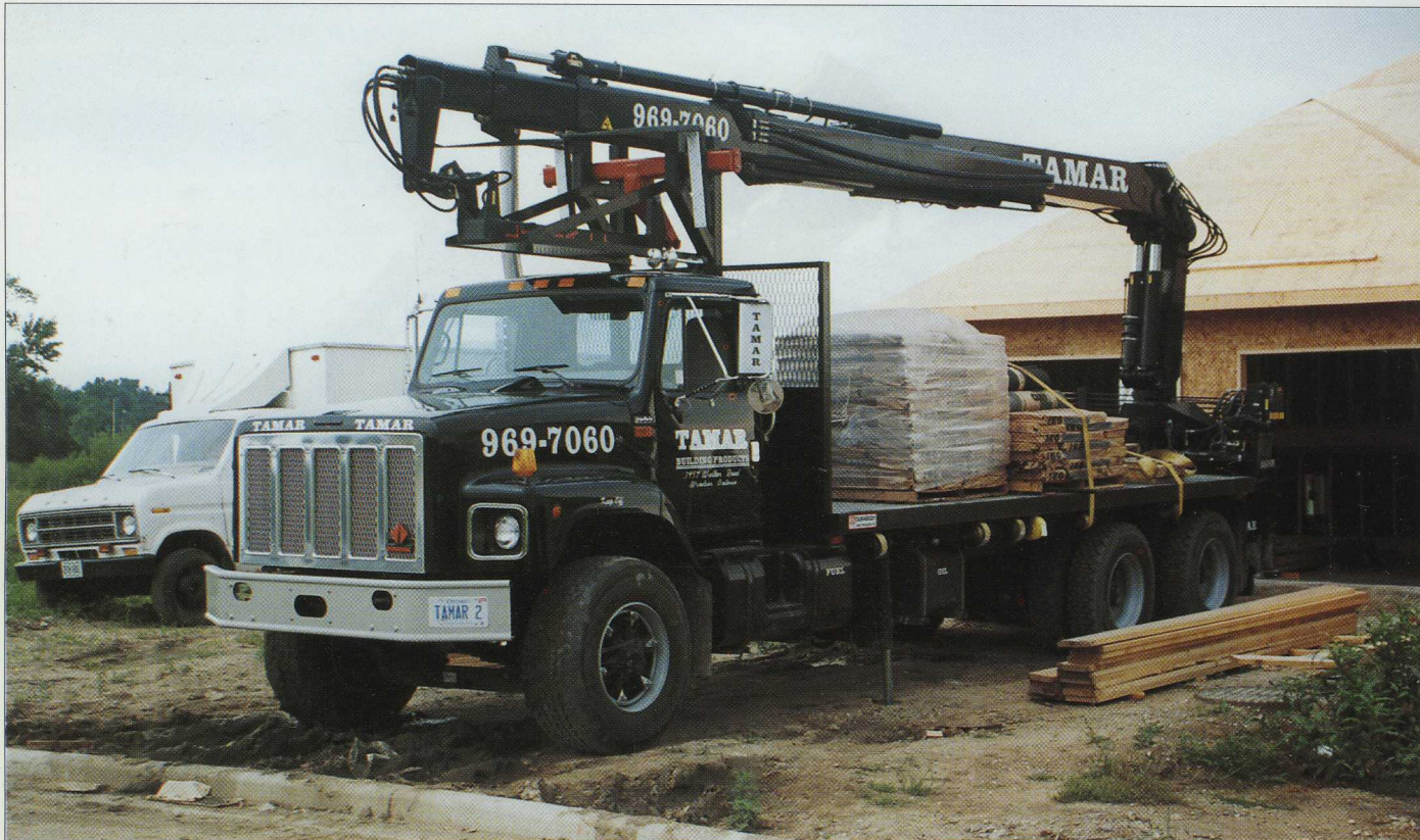
The HIAB 2650 has the new six-function HIAB Valve 50 which controls all boom movements as well as providing added overload protection.
