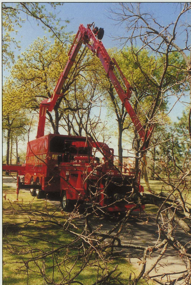
The Taylor's new HIAB 300-5 has a vertical reach of 92 feet (28 metres) and is equipped with remote control.
