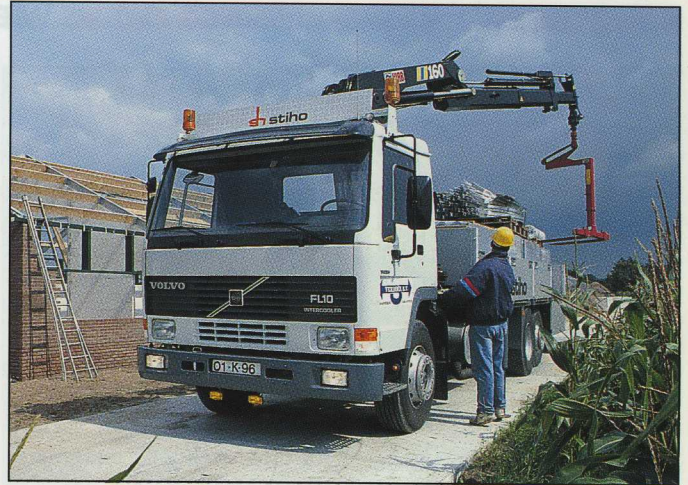
To deliver a wide range of materials, Verhoef B.V., a building supply company in Maarsse, a small town just northwest of Utrecht, uses a HIAB 160-3 equipped with a rotator and a fork. The crane's impressive hydraulic reach (10.4 metres) makes it easy to unload tiles, insulation, etc exactly where they're needed. And that is something customers are demanding today.
