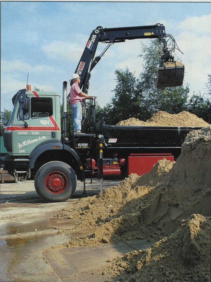
W. Herms and Sons, a family owned transport company in Epe, a small town in North Eastern Holland, use their new HIAB 105-2 equipped with a rotator and clamshell bucket primarily on contract jobs for the local municipal government. Specially designed for both cargo handling and bucket operation, the HIAB 105 features among other things an extremely compact boom system that allows a bucket to be easily stored on even a short truck bed.
