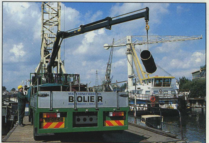
The HIAB 060 is one of the most popular cranes in its capacity class. And when equipped with a variety of accessories. It can be used for a wide range of applications - everything from handling building materials and machinery to installing electrical equipment and collecting waste. The HIAB 060-2 at the left, for instance, is a familiar sight in Apeldoorn where it makes its rounds daily to pickup, empty and distribute the bins that are used by the city's sanitation department to collect various kinds of recyclable waste materials. While Bolier Machinefabriek in Dordrecht, on the outskirts of Rotterdam, use their new HIAB 060 (above) to handle the marine engines they sell and service.
