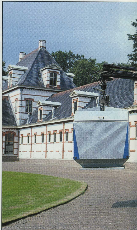
W. Herms and Sons, a family owned transport company in Epe, a small town in North Eastern Holland, use their new HIAB 105-2 equipped with a rotator and clamshell bucket primarily on contract jobs for the local municipal government. Specially designed for both cargo handling and bucket operation, the HIAB 105 features among other things an extremely compact boom system that allows a bucket to be easily stored on even a short truck bed.
