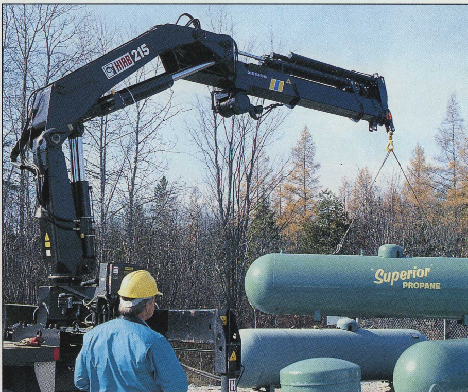
Gord Sloane is able to perform a wide range of jobs with his HIAB 215-4 which has a hydraulic reach of 11.7 metres.
