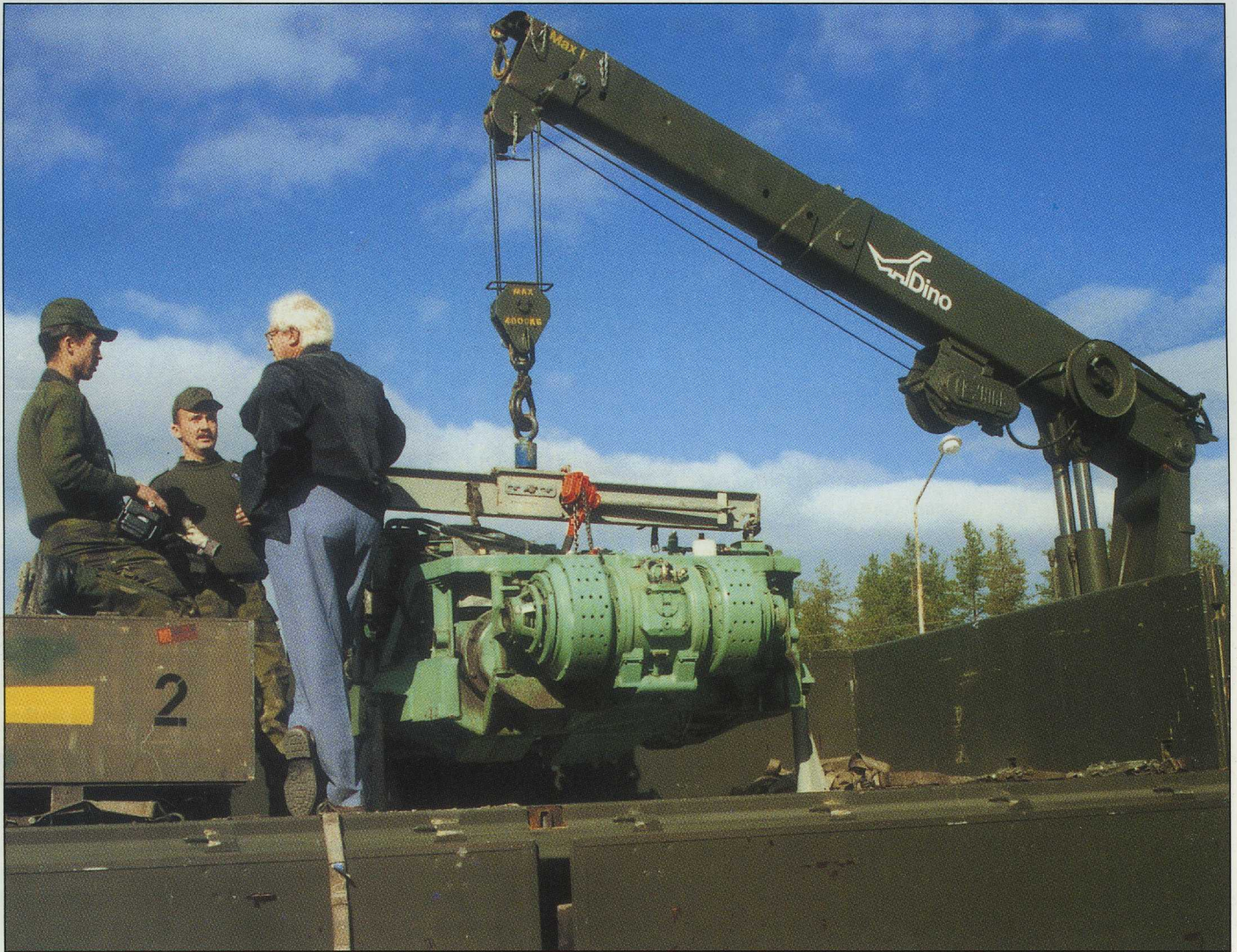
The HIAB 8801/3 has been specially designed to work as a supply crane for tracked, automatic 15.5 cm guns.
