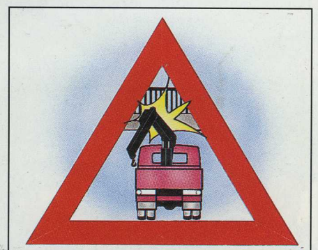
A warning signal sounds when the crane is not properly parked and this minimizes the risk of accidents.
