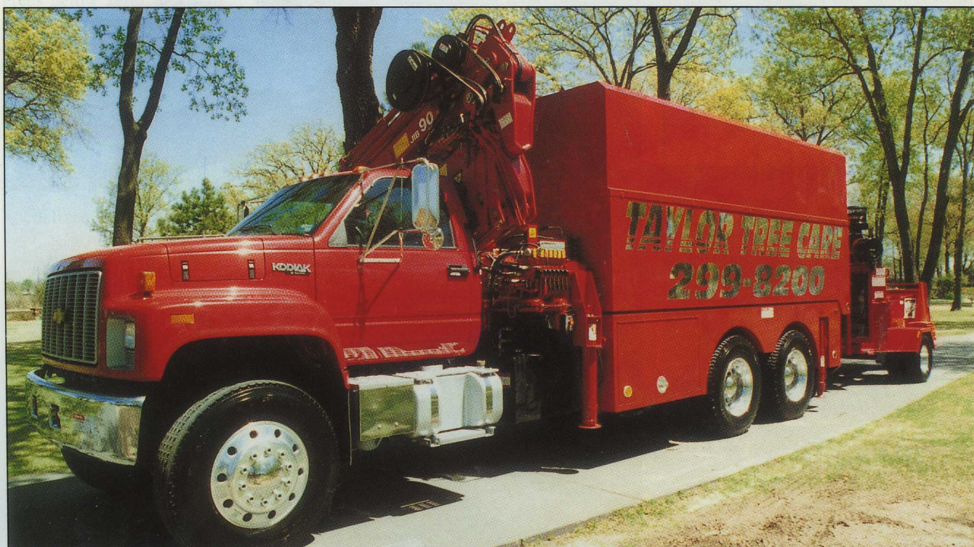
The crane is installed behind the cab leaving lots of room for a chip-box Gene Taylor designed himself.
