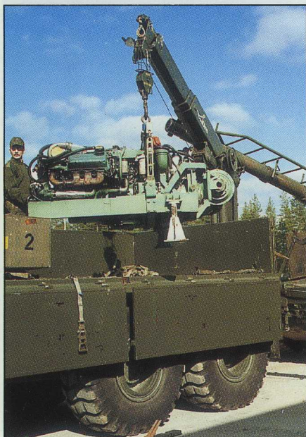
The crane is equipped with a remote control system for precision handling.
