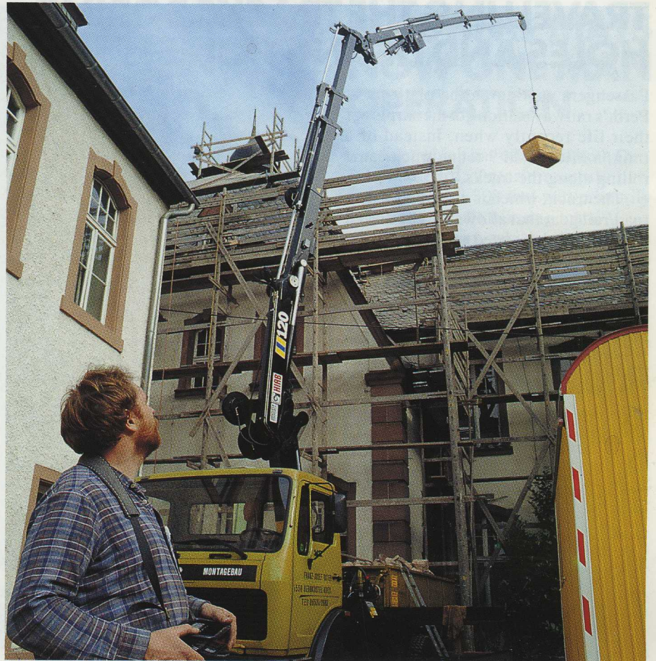
Mr. Oster's HIAB 120-2 is equipped with a winch, a jib and a Hiab remote control.
