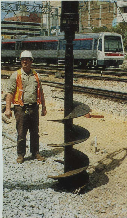
This HIAB 140 is equipped with a large earth auger.
