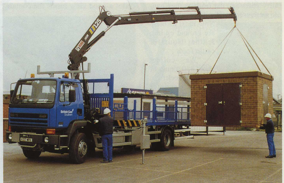
The versatile HIAB 125-3 can lift over 6,000 kg at a reach of 1.8 metres.
