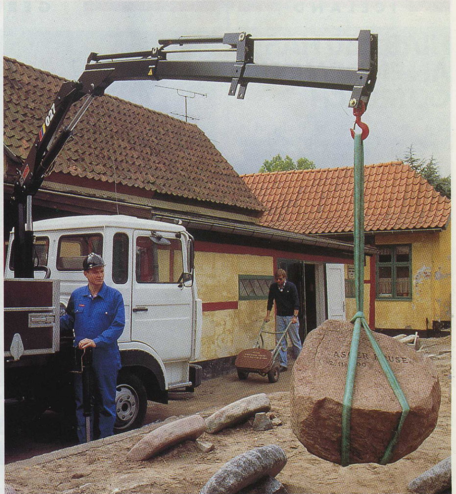
The HIAB 027 has a maximum hydraulic reach of 4.7 metres.
