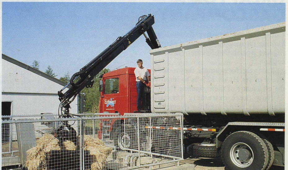
Euroveer's new HIAB 060-2 is mounted on a truck equipped with a demountable system.
