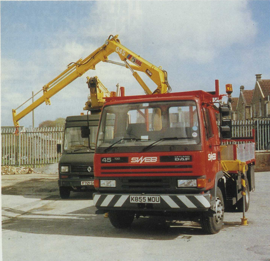
SWEB's HIAB 045-2's have a hydraulic reach of over six metres which makes them ideal for erecting and servicing light standards.
