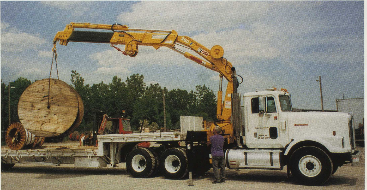
Ameritech uses their HIAB 260 AW almost exclusively for handling telephone cable reels.
