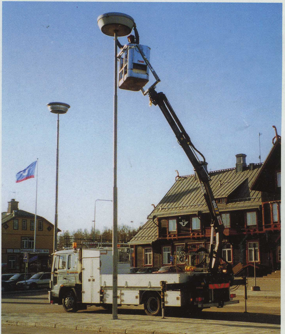
A Volvo FL 612 mounted with a HIAB 060 using the new LOGOS PB 250 personnel basket.
