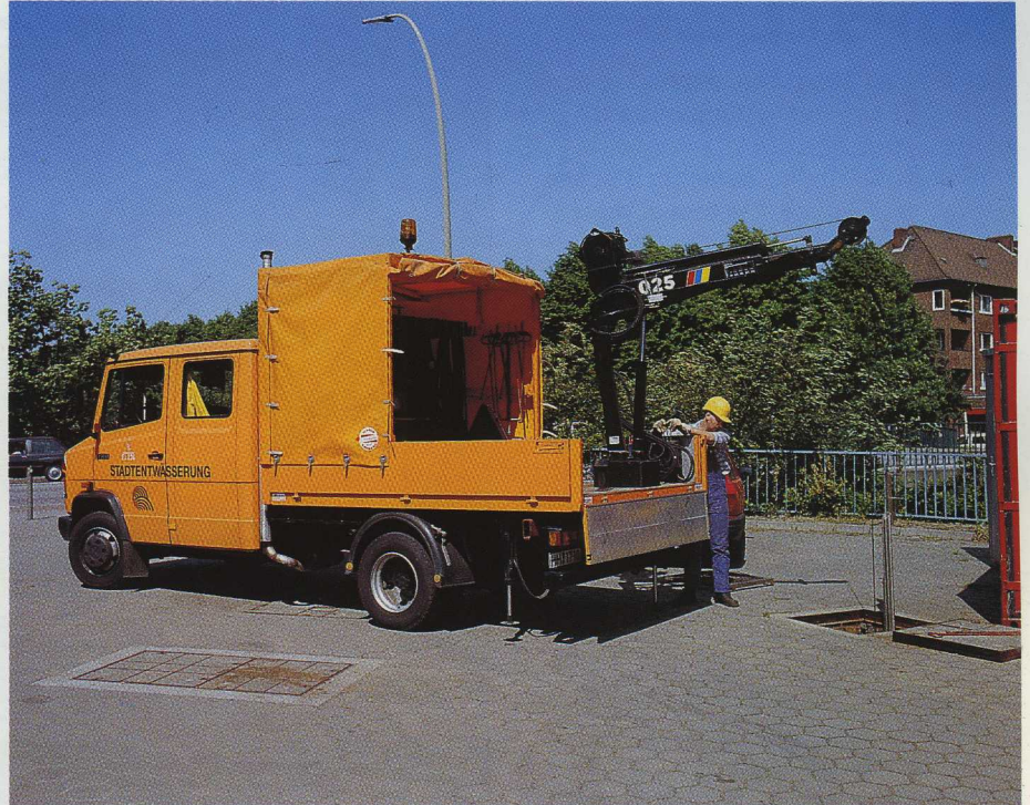
The HIAB 025 has a boom that reaches to almost 5 metres above the truck platform.
