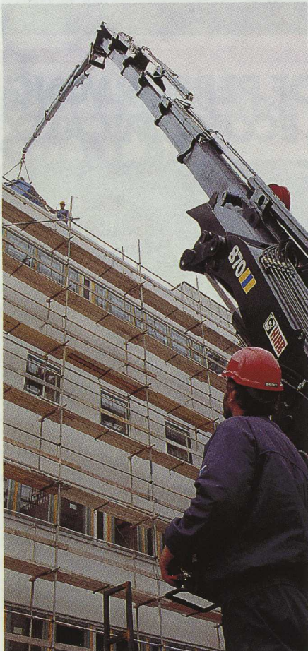
The new HIAB 870 has a lifting capacity of over eighty tonne-metres.
