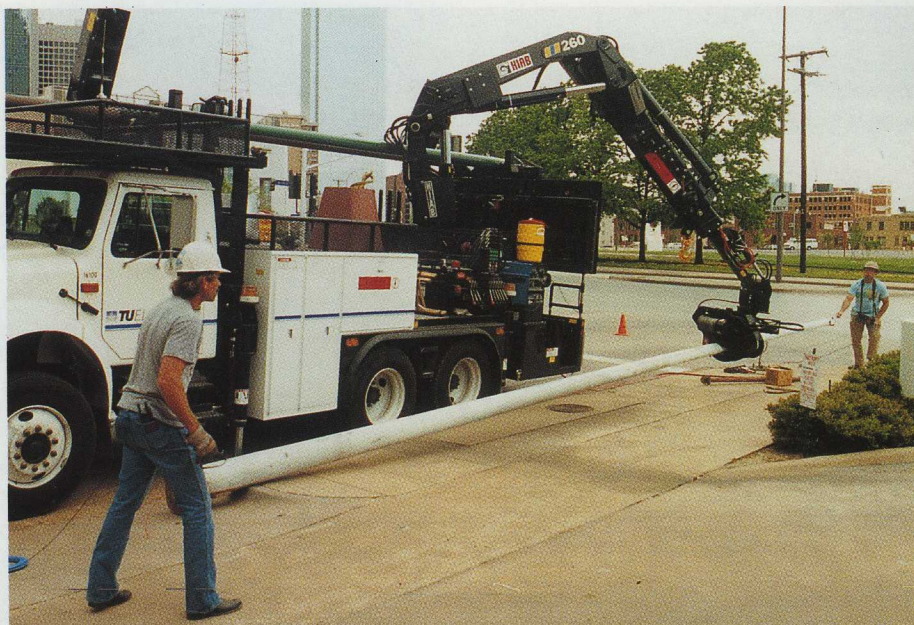
This HIAB 260AW has several hydraulic attachments.
