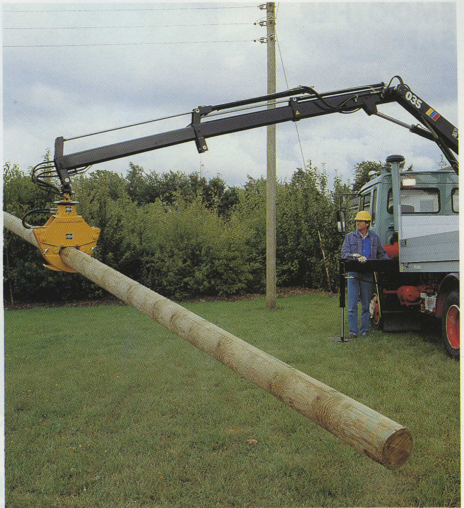
The new HIAB 035 has a maximum reach of over nine metres.
