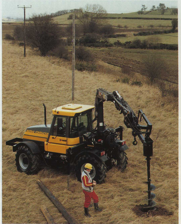
To provide extra flexibility in a variety of applications, Hiab cranes are being installed on a lot of Fastracs in England.
