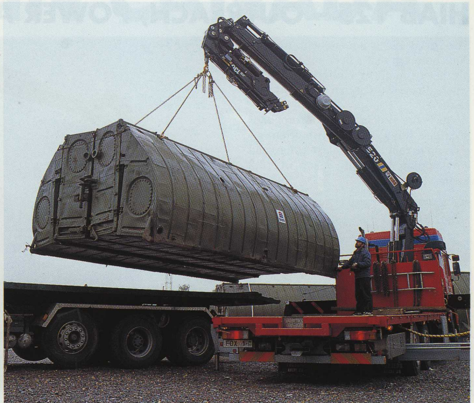
This new 52 tonne-metre crane has a lifting capacity of over 3.3 tonnes at a reach of nearly 14 metres.
