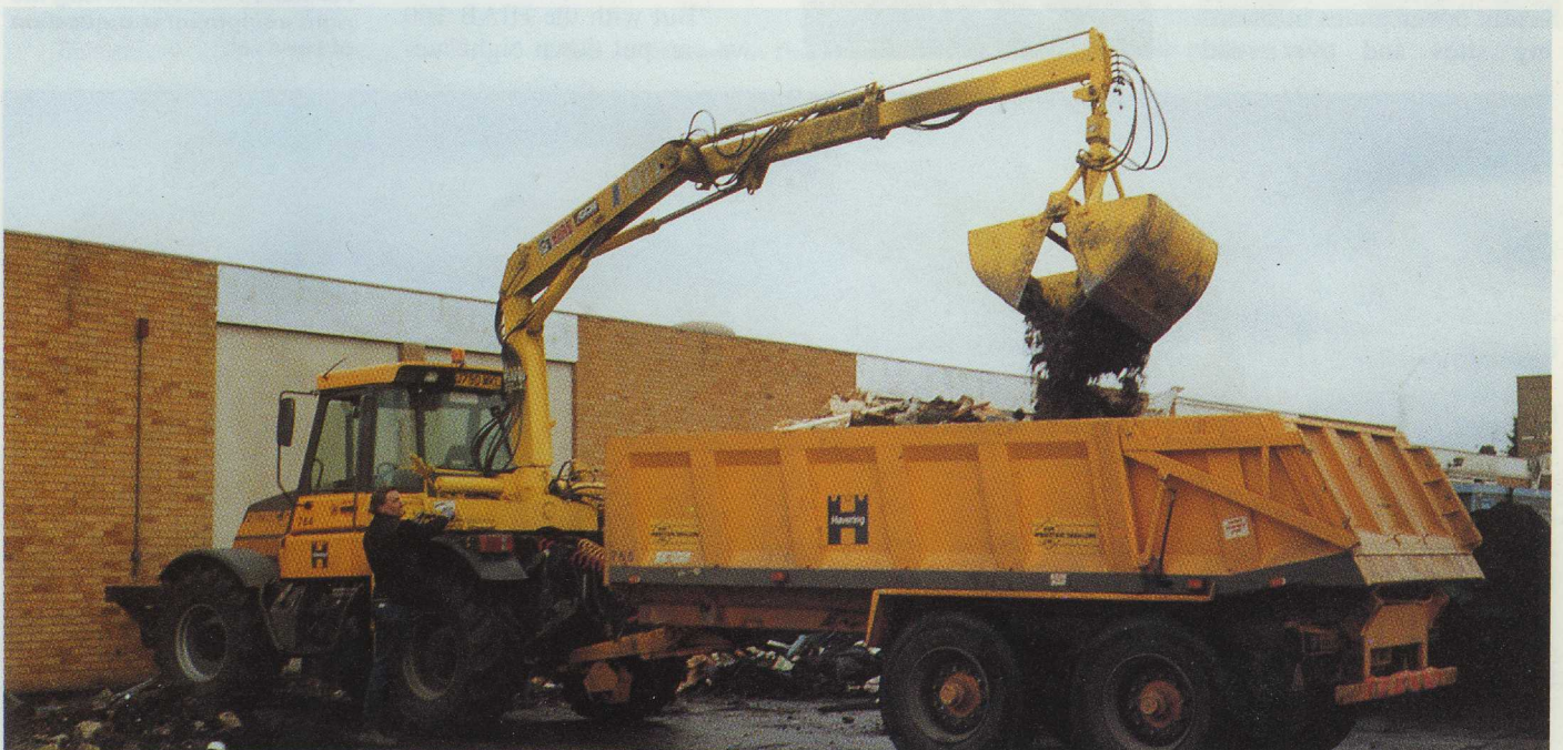
The London Borough of Havering's new Fastrac 125 fitted with a HIAB 071.
