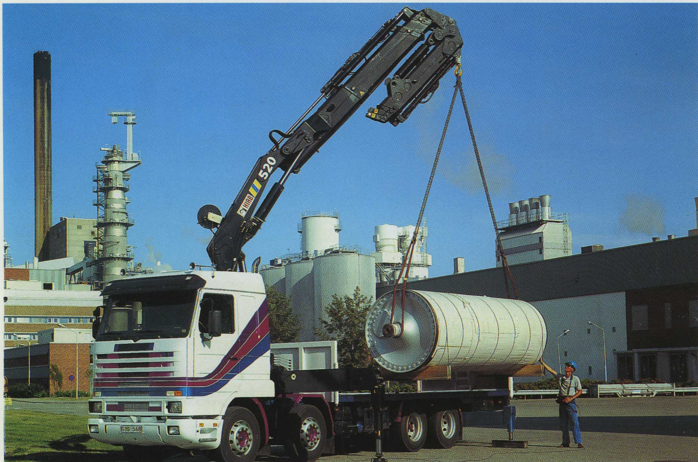
The HIAB 520 has hydraulically operated outrigger extensions with a span of up to seven metres.
