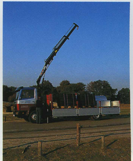
With two manual extensions, the HIAB 045's reach can be extended to over 10.5 metres.
