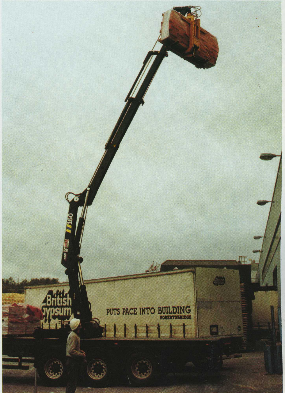
This HIAB 160-3 has been mounted so as to allow the trailer's full payload potential to be economically utilized.
