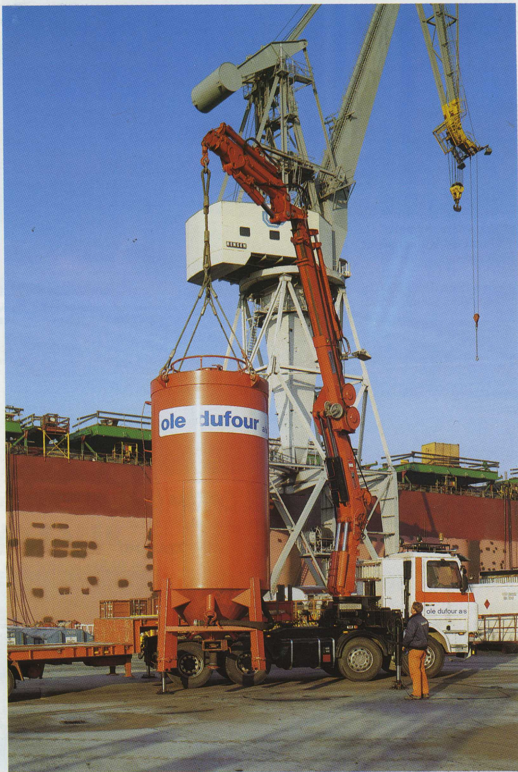
Ole Dufour Ltd.'s HIAB 450 has a reach of 22.5 metres.
