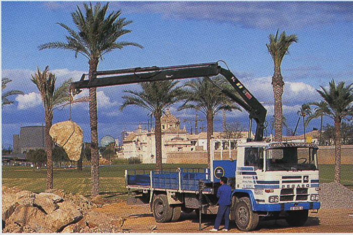
Silverio Ramirez (right), the owner of Silverio Transport S.L., has been in business in Seville for almost 18 years. He uses his HIAB 140 AW mounted on a two-axel Pegaso for loading and unloading a variety of building materials. One of Silverio's drivers (above) removing large boulders from a lawn. In the background are the monastery and ceramics factory which until recently were the only buildings on the Isla de la Cartuja, the site of EXPO '92.
