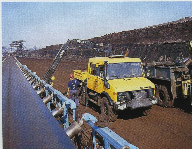
Several HIAB's mounted on Unimogs are used to handle a variety of equipment.
