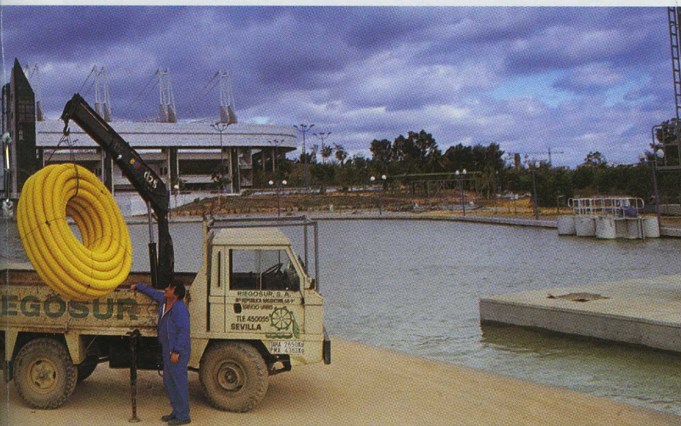
Riegosur S.A. , a landscaping company in Seville (left), is responsible for installing most of the sprinkling and irrigation systems for the more than 500,000 sq. metres of parks and gardens at EXPO '92. To make their job easier and more efficient they had a HIAB 025-2 installed on an old Land Rover Santana.
