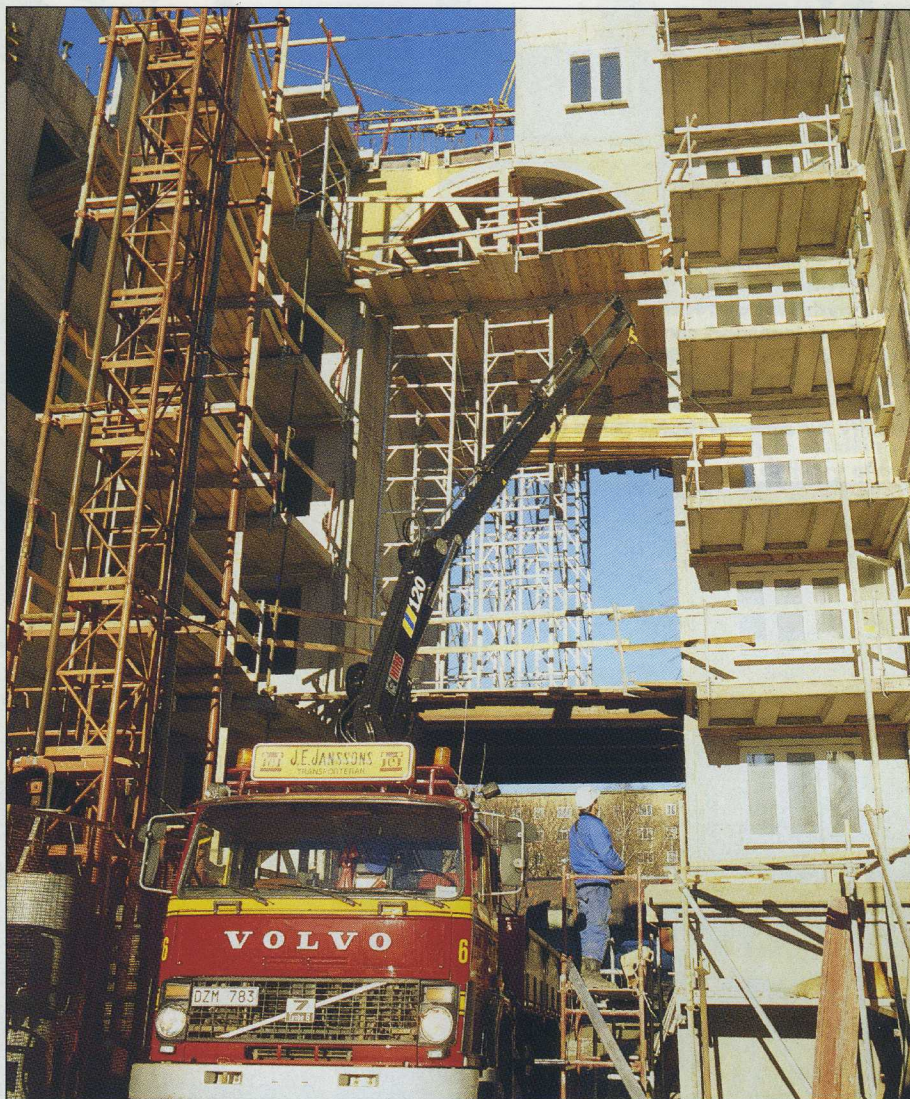
This is a HIAB 120-3. But the HIAB 120 also comes with up to four hydraulic extensions.
