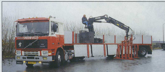
Rol-loaders are perfect for handling bricks and blocks.
