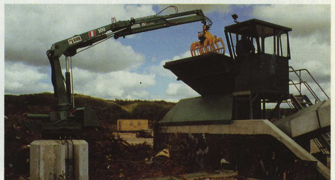
This stationary HIAB 100 AW/B3 is used in Denmark to sort objects that can't be burned from household waste.
