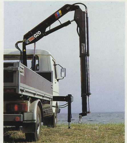
The HIAB 020 has a working range of 5.7 metres with an optional extension.
