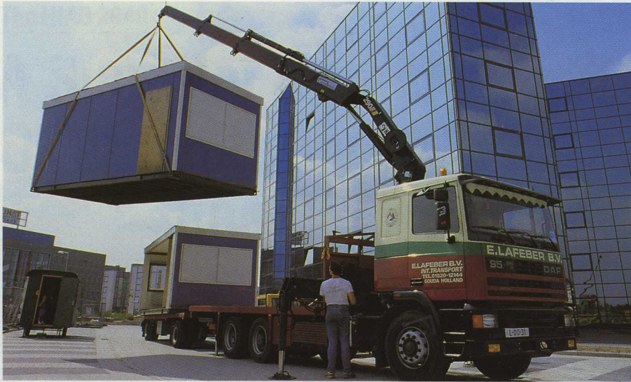
Raymond Ekkelboom unloads a workers' hut with Lafeber's new HIAB 290.
