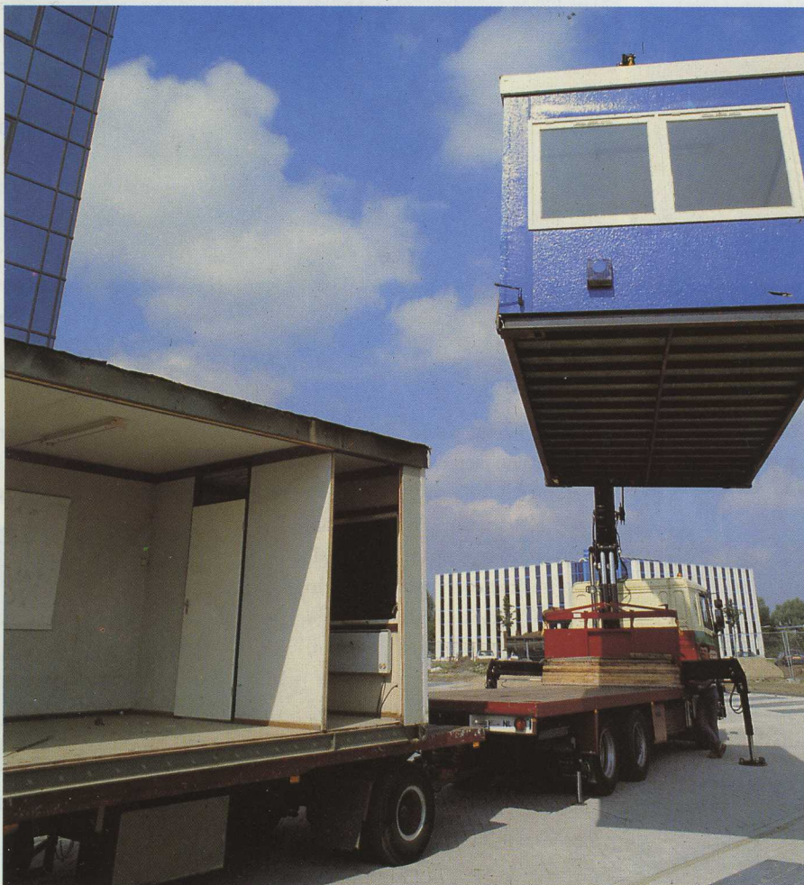
The recently patented HIAB LOS (Load Operated Speed) function on the new HIAB 290 makes material handling safer and increases lifting capacity by 10 to 15%.
