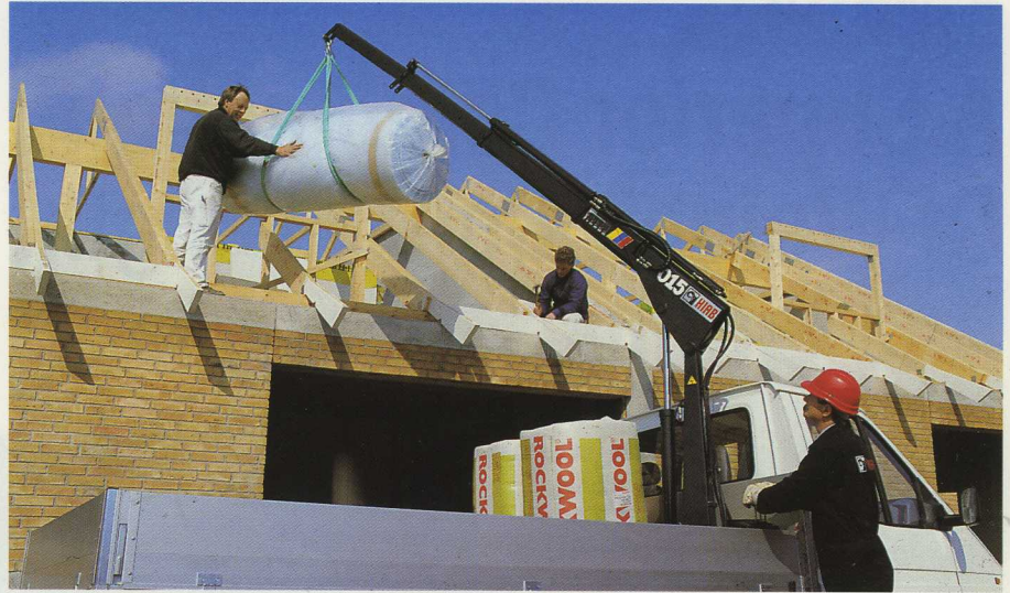
The HIAB 015 is probably the most compact 1.5 tonne metre crane ever built.
