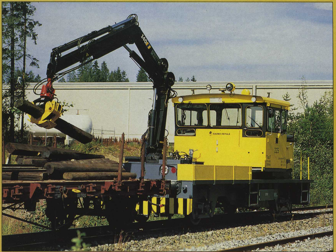
A sleeper grab is one of the many hydraulic attachments that are employed with the HIAB 140 when it is mounted on a Rail Truck.
