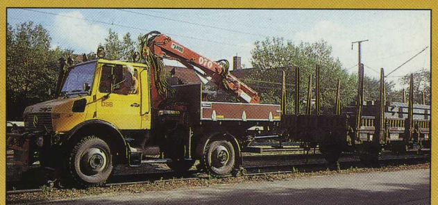
A towbar turns the vehicle into a small shunting engine. The coupling is operated from the driver's cab.
