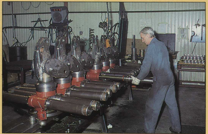
The FMV 290 has a slewing system featuring double hydraulic cylinders in an oil bath. Seen here is the assembly of the short-king post version.
