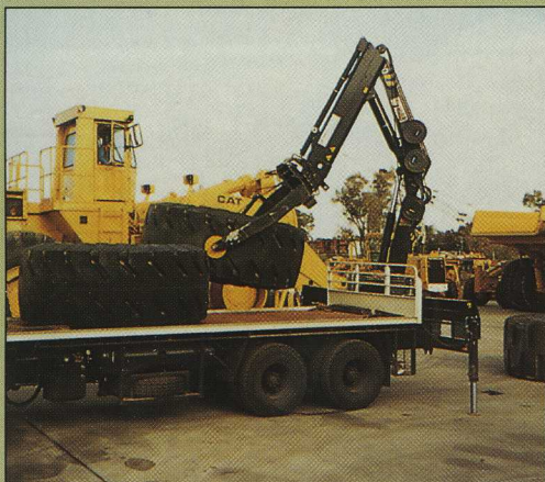
This close-up brings home the impressive dimensions of both the tyre and the grab. The latter was designed by HIAB-FOCO's general agent in Australia.
