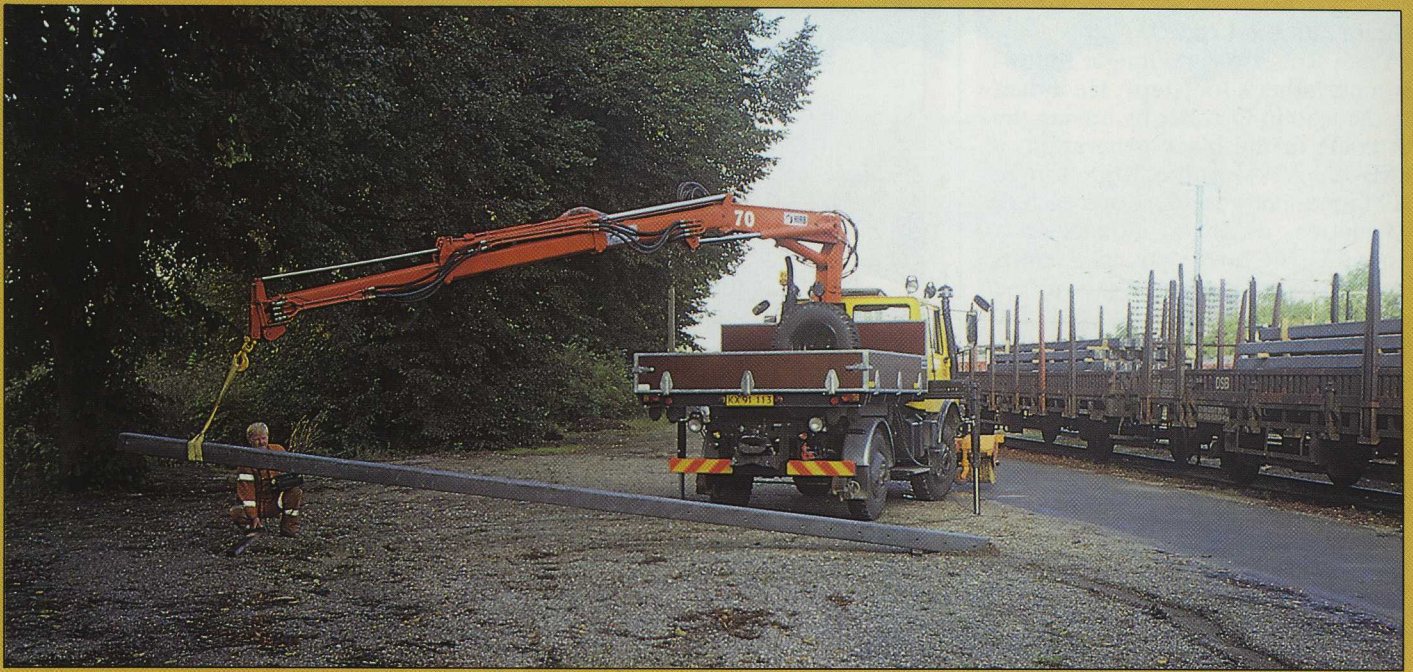
Using a DigiDrive the operator can control the crane from a position right next to the load.
