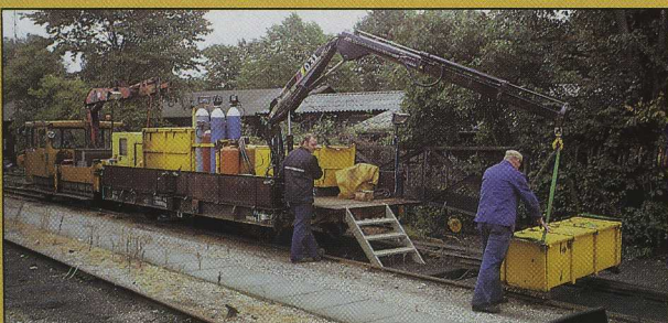
The HIAB 031 handles tool-boxes, gas cylinders and other equipment used in maintenance work.
