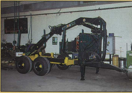
An FMV 240 with a hydraulic extension on a hydrostatically driven 9-tonne truck – a high-capacity combination for small-scale professional forestry.
