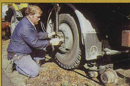
The suspension of the roadwheels is locked so as to firm the vehicle up when operating on the track.
