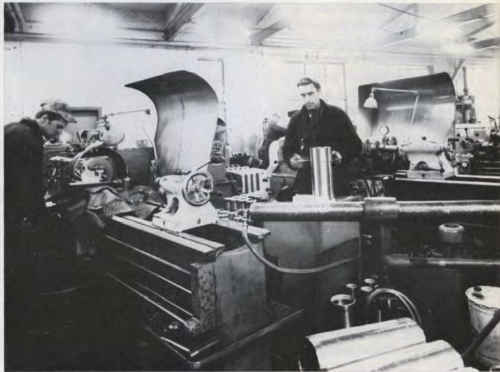
The pressure-rolling of the cylinder surfaces is a job that has a decisive influence on the quality of the products. This is Gösta Forss, checking the tolerances and surface fineness of a newly rolled cylinder.
