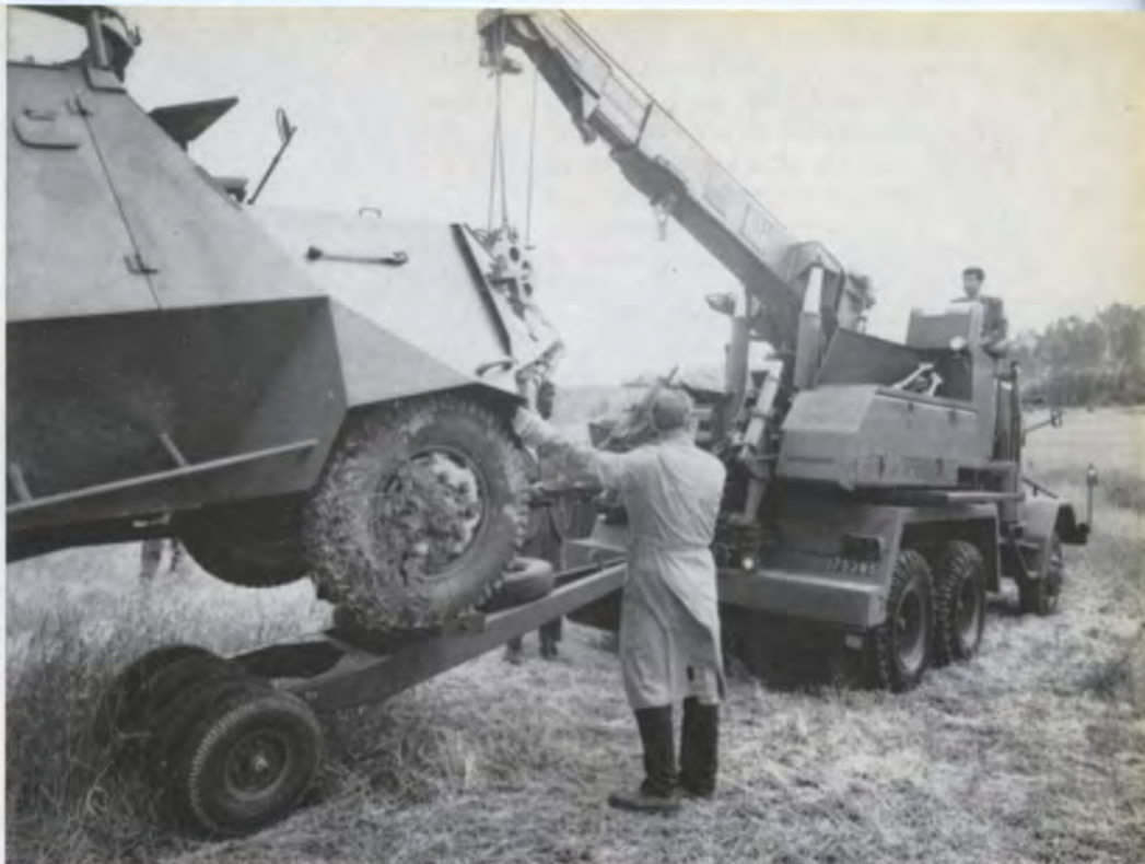
With a 10-ton lift packed in its crane the new rescue truck has no trouble with this personnel carrier, despite the dead weight of its armour plate.
