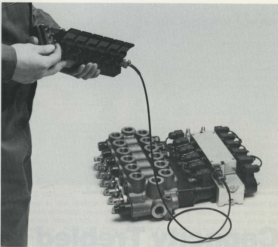
In the DigiDrive, outgoing signals from the controller are transmitted through a cable to an actuator mounted on the control valve.
