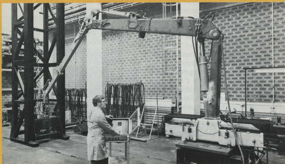
A fatigue test on a Jonsered 700.
