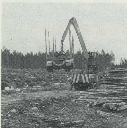
The trailer, weighing 7.3 tonnes, is "side-tracked" so that the tractor truck can back up and be loaded.
