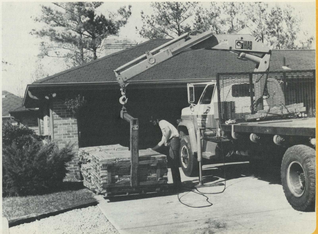
With the HIAB Method the unaided driver can get through from six to eight drops a day. Remote control reduces the risk of damage.
