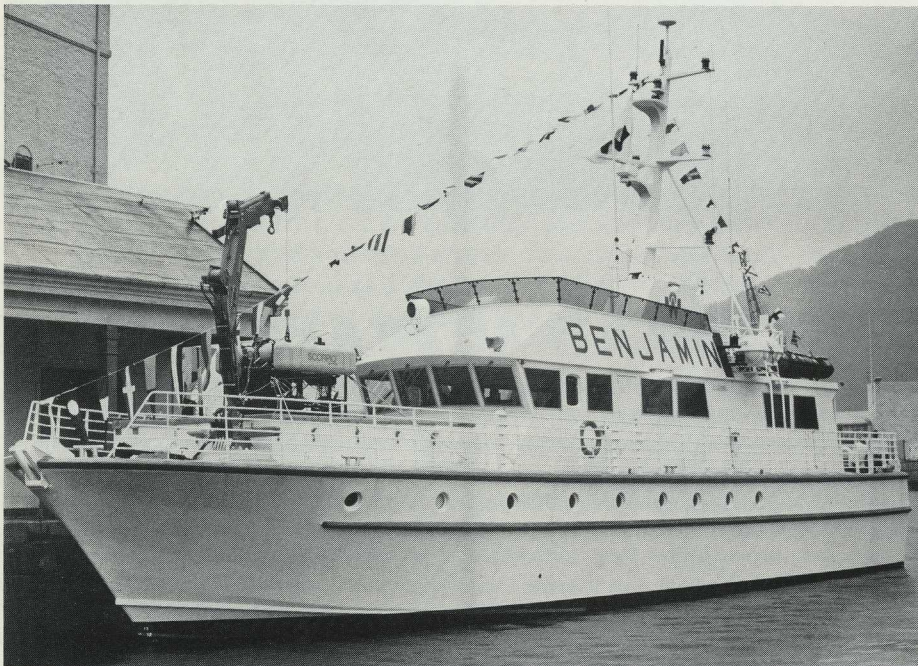
The M/S "Benjamin", which is to be based in Bergen, is a 114-tonner capable of 20 knots. It has room on board for twelve people.
