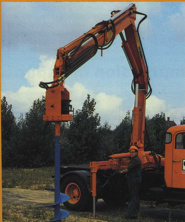
The earth auger, a very effective implement, will easily and speedily make holes for posts, plinths, flagpoles and so on.
