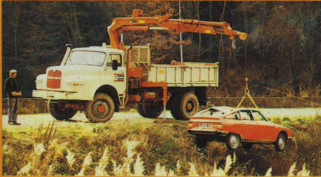
The winch is a very versatile accessory that greatly increases the utility of the crane.
