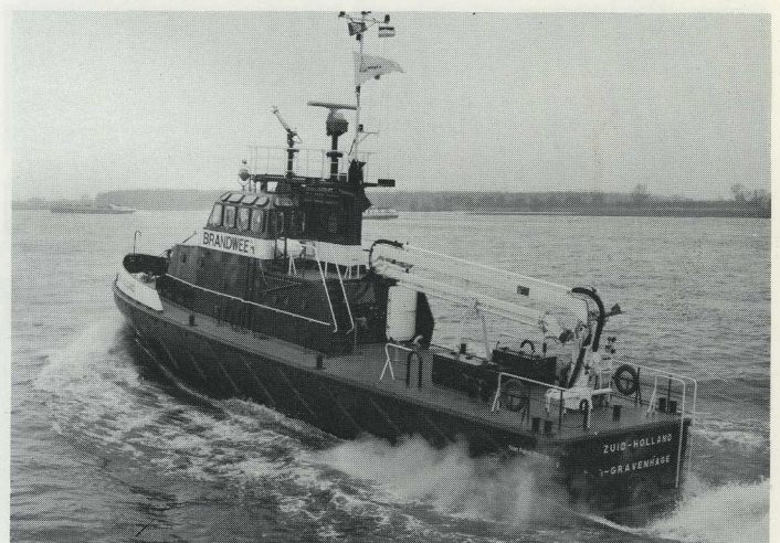
A close-up of the crane in the parked position on the stern deck of the ship. The crane is operated either from the stern deck or with the aid of a HIAB EMPROC from the wheelhouse.
