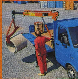
With a culvert hook it's no trouble to handle heavy, unwieldy concrete well-casing sections.
