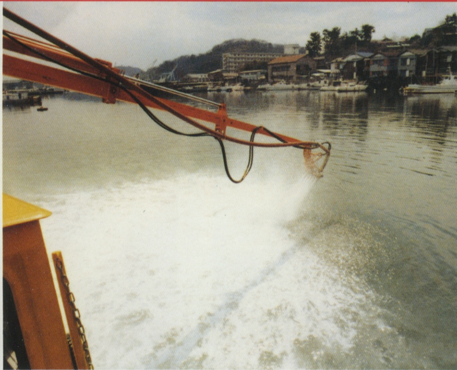
The water projected from the jet nozzle, which is handled by the HIAB crane, flushes floating litter towards the intake of the sweeper vessel.
