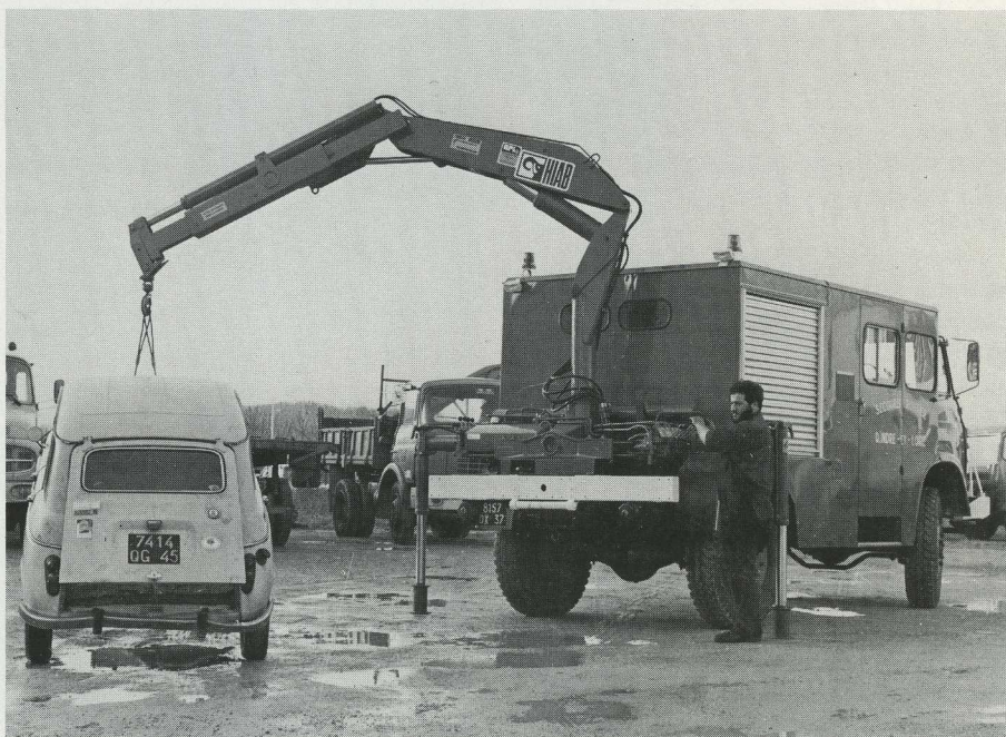
The emergency truck of the fire brigade in Tours has a HIAB 650 AW and a water tank among other equipment, along with room for a six-man rescue team.
