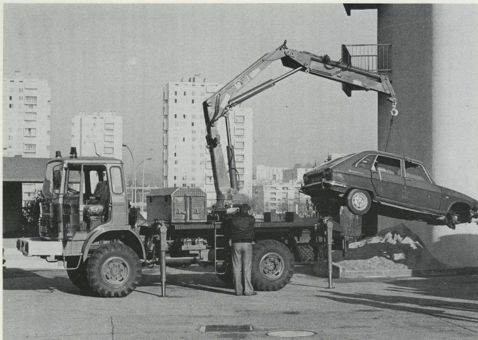
The new emergency truck in Limoges, which is equipped with a HIAB 1165 AW, can do a great many other jobs besides recovering cars.
