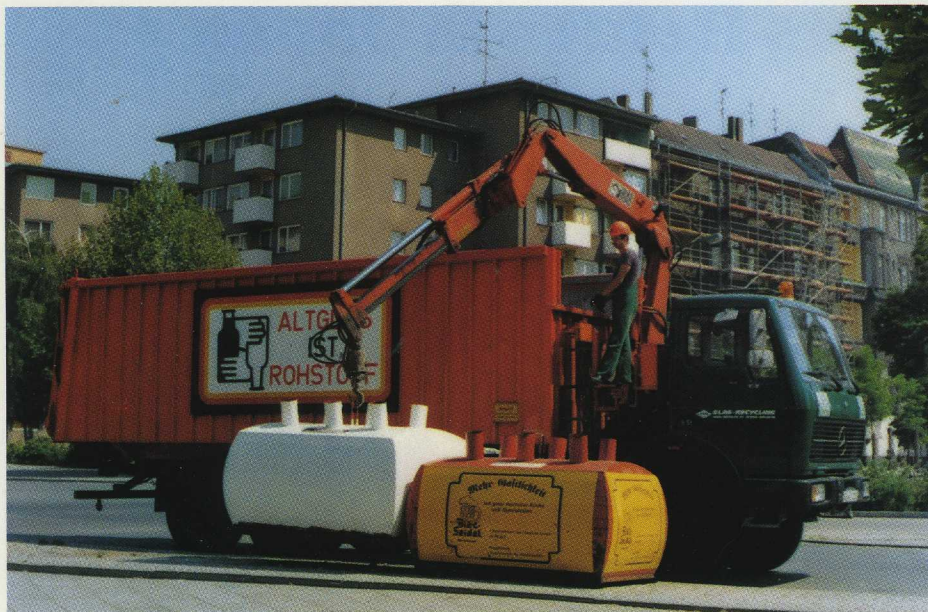
In Berlin the waste-glass containers are handled by a HIAB 850 AW, controlled from a platform at the crane base.
