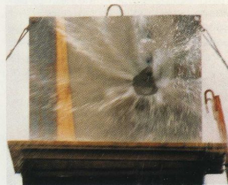
The drill has broken through the wall and water is squirting in all directions on the "inside". Below is a close-up of the drilling unit with its 110-mm concrete drill.
