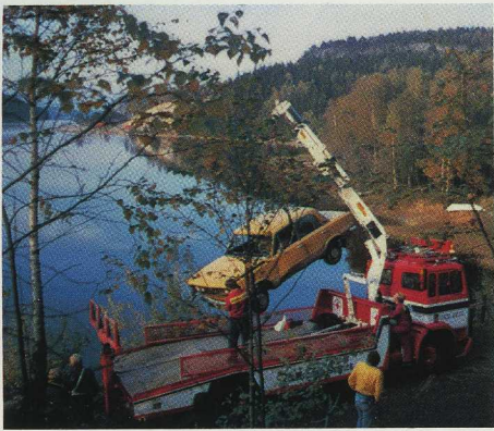
Cars that have gone to the bottom of a lake or plunged down one of the many steep banks along this stretch of road are best recovered by the HIAB Method.
