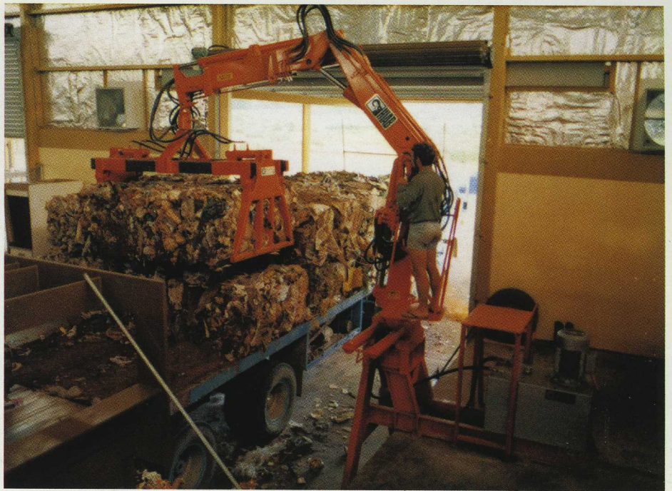
Within three weeks the HIAB experts beat the problem of the waste bales and set up the HIAB shown on the right, which lifts two bales at a time using the above grapple.
