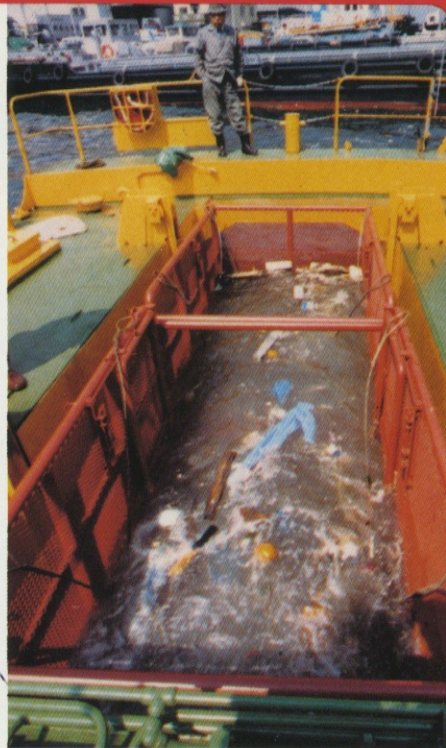
Rubbish and contaminants are collected in a mesh container, which can be replaced by an empty one as soon as it is full.
