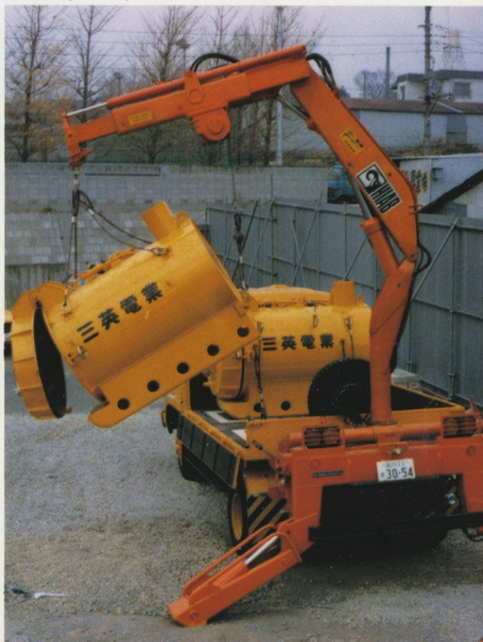
If the sludge is not pumped over into the tanker truck the tanks can be emptied with the aid of the crane and the winch, which are hooked up to straps at the rear end of the container.
