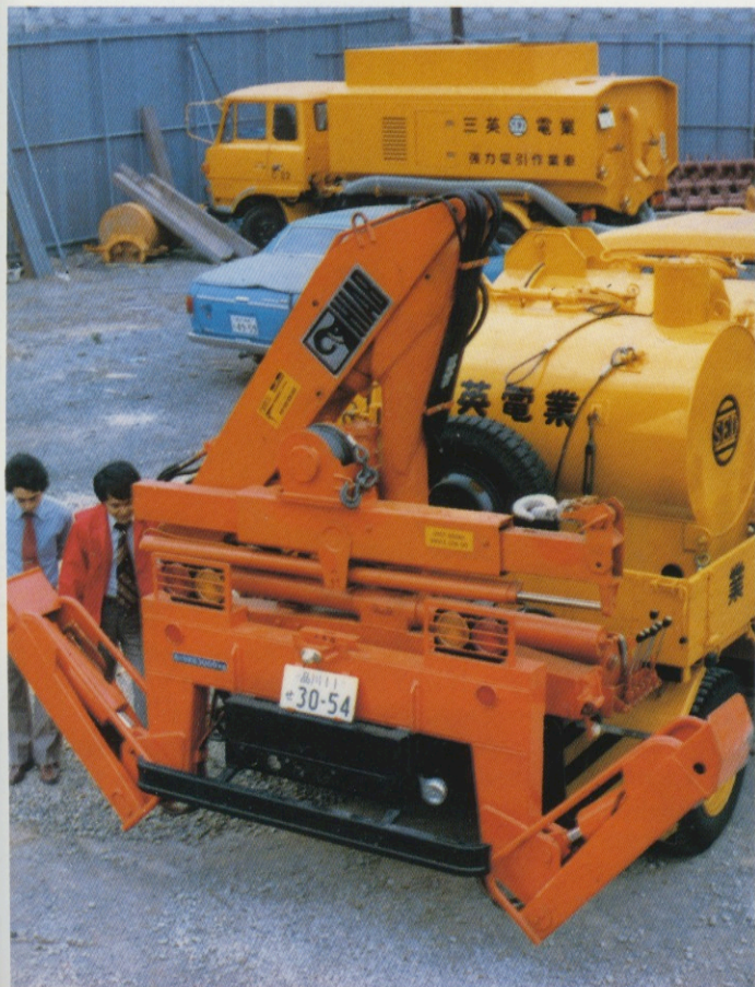
In the foreground is the suction vehicle, with its HIAB 650 and its flap-down support legs. In the background is the tanker truck.
