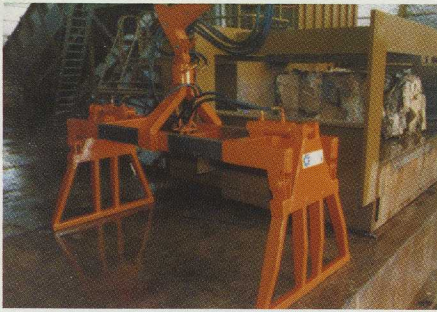
Within three weeks the HIAB experts beat the problem of the waste bales and set up the HIAB shown on the right, which lifts two bales at a time using the above grapple.
