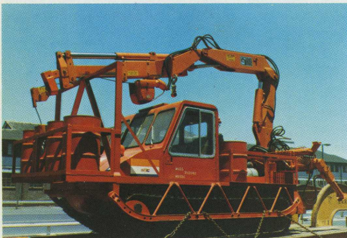
The HIAB mounted on one of the crawler tractors, ready to be loaded aboard ship.
