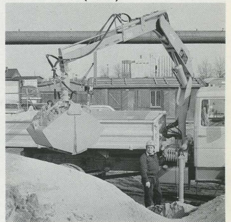
A new control valve, the HIAB 31 (above), gives smoother loader movements, and a double-acting inner-boom cylinder makes the machine more effective for attachments like the sand bucket (below).
