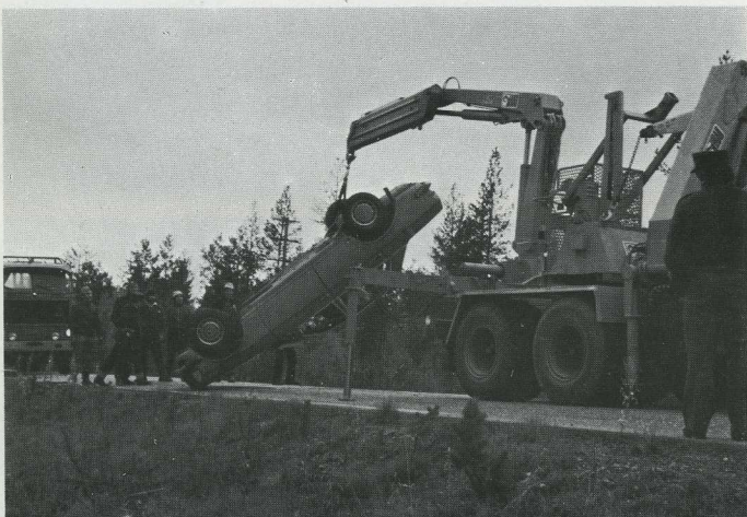
Help has arrived. A truck mounting half-a-dozen HIAB loaders makes short work of most obstructions. Lifting a car clear is a cinch for the HIAB 965.
