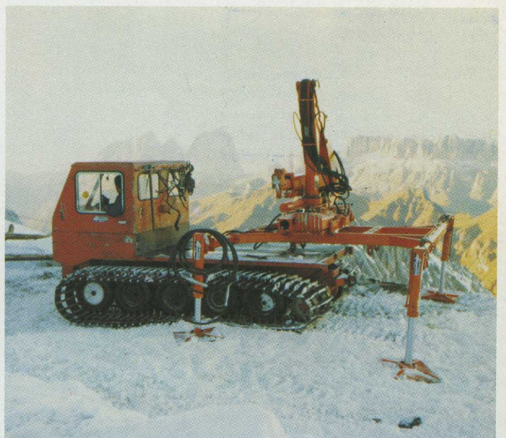
The lightweight frame can easily be laid off on the support legs so as to release the crawler tractor.
