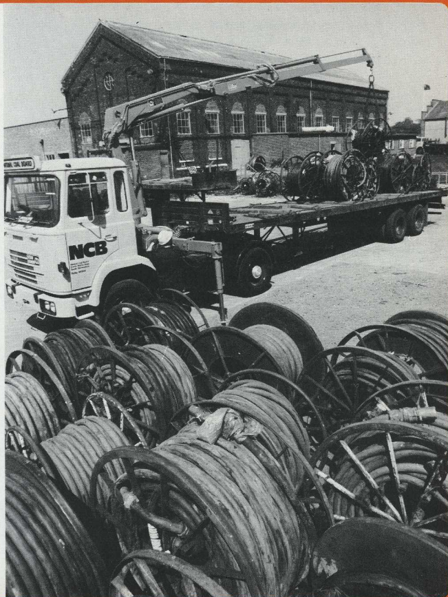
South Coast Welders Ltd. built themselves a mobile crane using a HIAB 1165, and the design turned out so well that they're now planning to produce it for sale.
