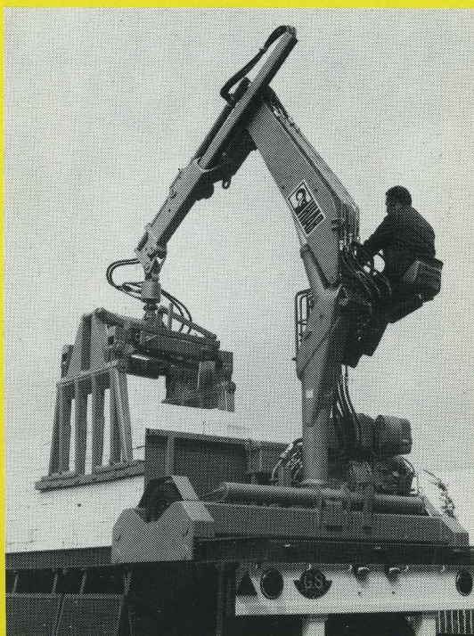
(Left:) A HIAB 650 as a Rol-loader, with top-seat controls and a brick clamp. (Below:) The drive mechanism, with the hydraulic motor and the transmission. (Right:) The controls, the diesel engine that powers the unit, and the stout support- and drive-wheels.
