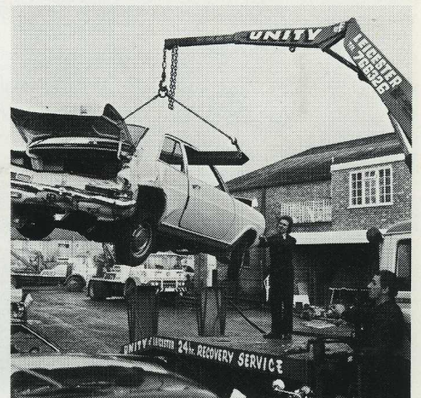
A car has gone off the road and buried itself in the soft, wet verge. Dragging it clear with a winch would cause still more damage to the vehicle, the ground and the hedge. The HIAB crane lifts it onto the transporter without further harm. It will soon be fully roadworthy again.
