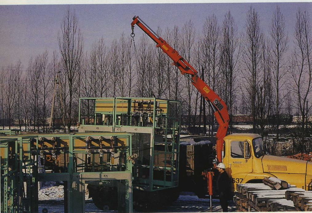
The state enterprise ELBUD builds the high-tension lines that criss-cross Poland. It does much of its materials handling by the HIAB Method. These pictures show the loading of pipes onto a Fiat/Unic by a HIAB 550 (above) and of transformers (below).
