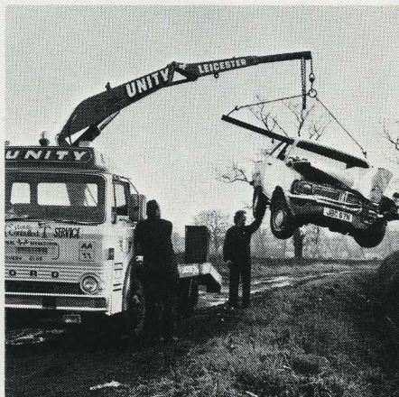
A car has gone off the road and buried itself in the soft, wet verge. Dragging it clear with a winch would cause still more damage to the vehicle, the ground and the hedge. The HIAB crane lifts it onto the transporter without further harm. It will soon be fully roadworthy again.
