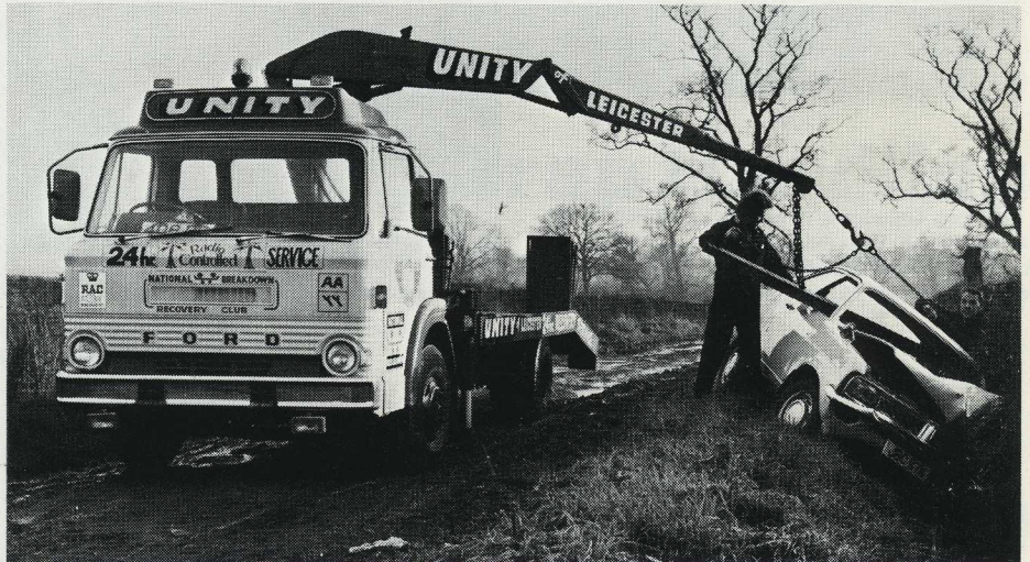
A car has gone off the road and buried itself in the soft, wet verge. Dragging it clear with a winch would cause still more damage to the vehicle, the ground and the hedge. The HIAB crane lifts it onto the transporter without further harm. It will soon be fully roadworthy again.
