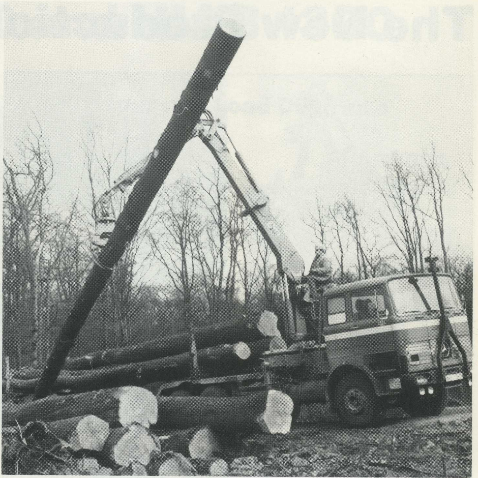
(Right:) A HIAB 1300 for whole-stem loading. The picture at the foot of the page shows a moment of peak exertion - the trunk being swung up with the aid of the cross-bar on the inner boom.
