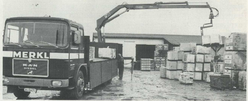
The double hydraulic extension of the "AW" version gives a standard reach of no less than 8.45 metres.
