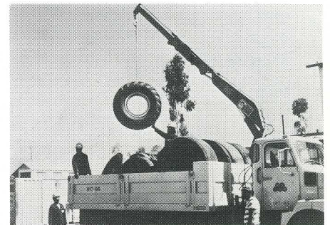
At Arequipa in southern Peru, tyres and other equipment for contracting machines are handled by a HIAB 550 (above). The cable reel on the left weighs 2 tons and provides a test-lift for the loader after an overhaul in Chiclayo. The tractor below, with its HIAB 550, is used for erecting power-line posts in the desert between Chimbote and Trujillo.
