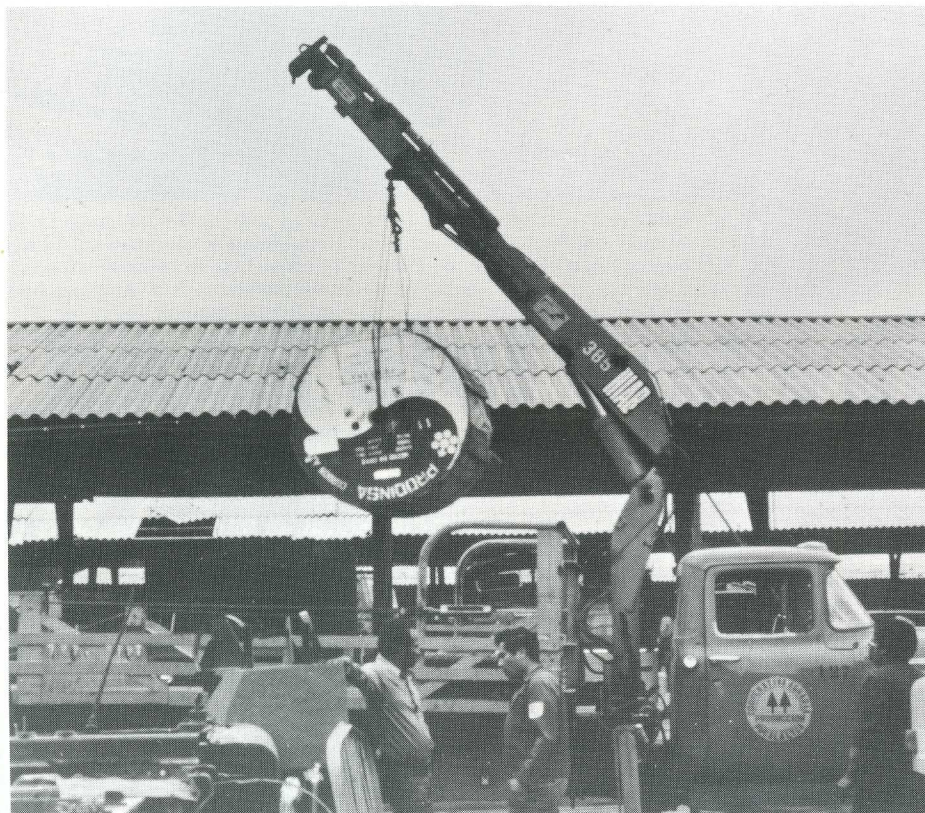
At Arequipa in southern Peru, tyres and other equipment for contracting machines are handled by a HIAB 550 (above). The cable reel on the left weighs 2 tons and provides a test-lift for the loader after an overhaul in Chiclayo. The tractor below, with its HIAB 550, is used for erecting power-line posts in the desert between Chimbote and Trujillo.
