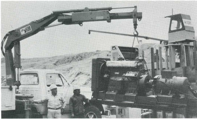
All the heavy equipment at an oil refinery in Bayovar, like this 2.5-ton diesel set, is handled by a HIAB 950 (above). On the right, a HIAB 950 hoists a transformer in Oroya. A HIAB 550 with a personnel basket (below) is used by the electricity works in Chiclayo for such tasks as cleaning insulators.
