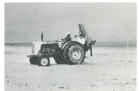
At Arequipa in southern Peru, tyres and other equipment for contracting machines are handled by a HIAB 550 (above). The cable reel on the left weighs 2 tons and provides a test-lift for the loader after an overhaul in Chiclayo. The tractor below, with its HIAB 550, is used for erecting power-line posts in the desert between Chimbote and Trujillo.
