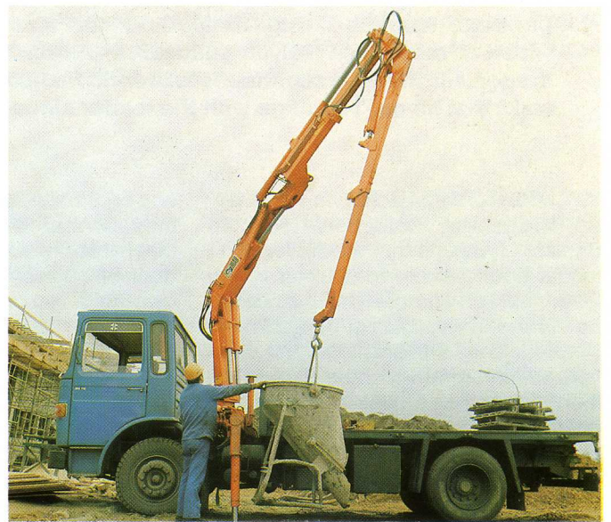
The extra hinge facilitates work close to the loader body.
