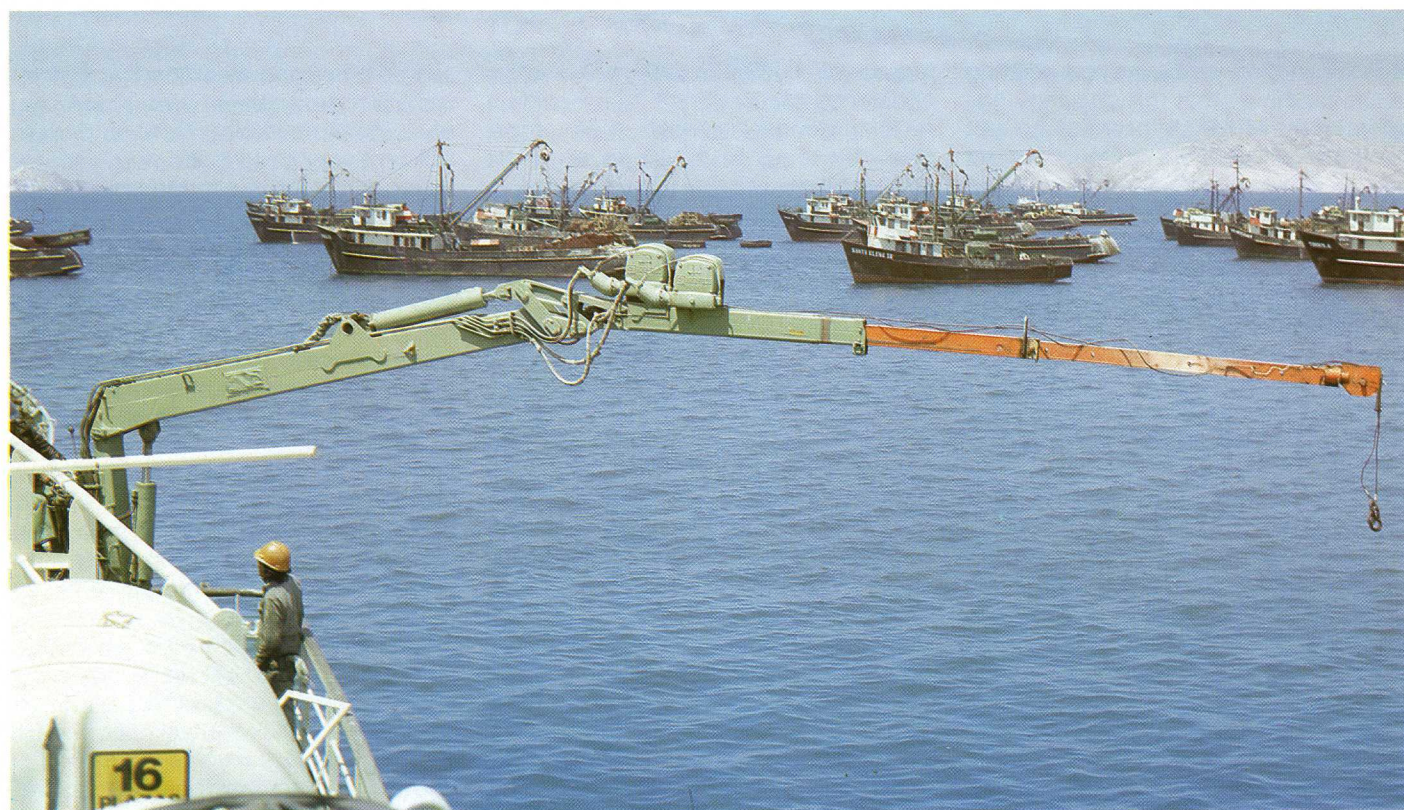
In the port of Chimbote in northern Peru the Picsa yard builds boats for the tuna fisheries and equips them with HIAB 670s. This one has double winches.
