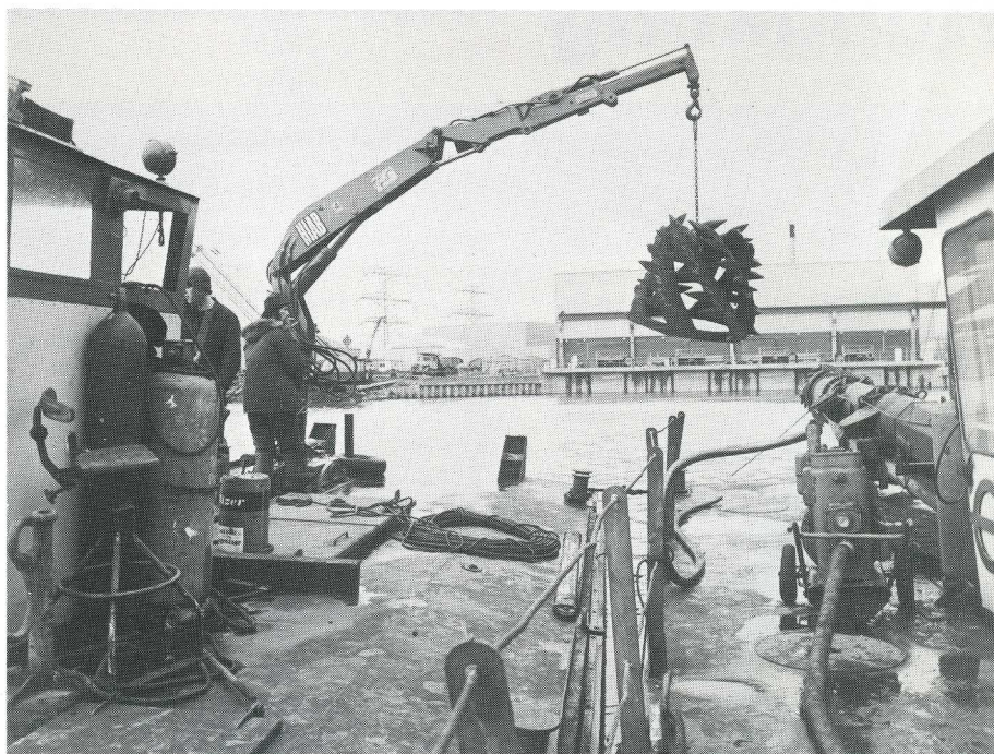
Handling the "Otary's" equipment is another assignment providing plenty of scope for the HIAB, seen here lifting one of the cutters that churn up material from the bottom so that it can be sucked in by the dredger.
