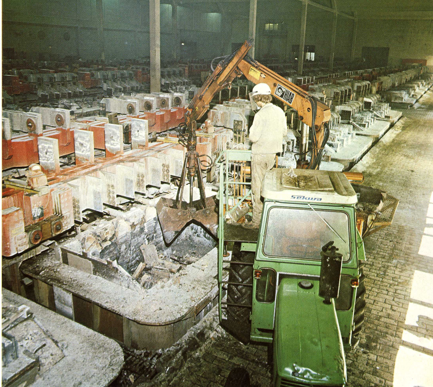
Slag and pieces of the old lining are scooped out of the electrolytic cell by the HIAB. The use of an elongated bucket keeps the hydraulic hoses well clear of the hot slag.
