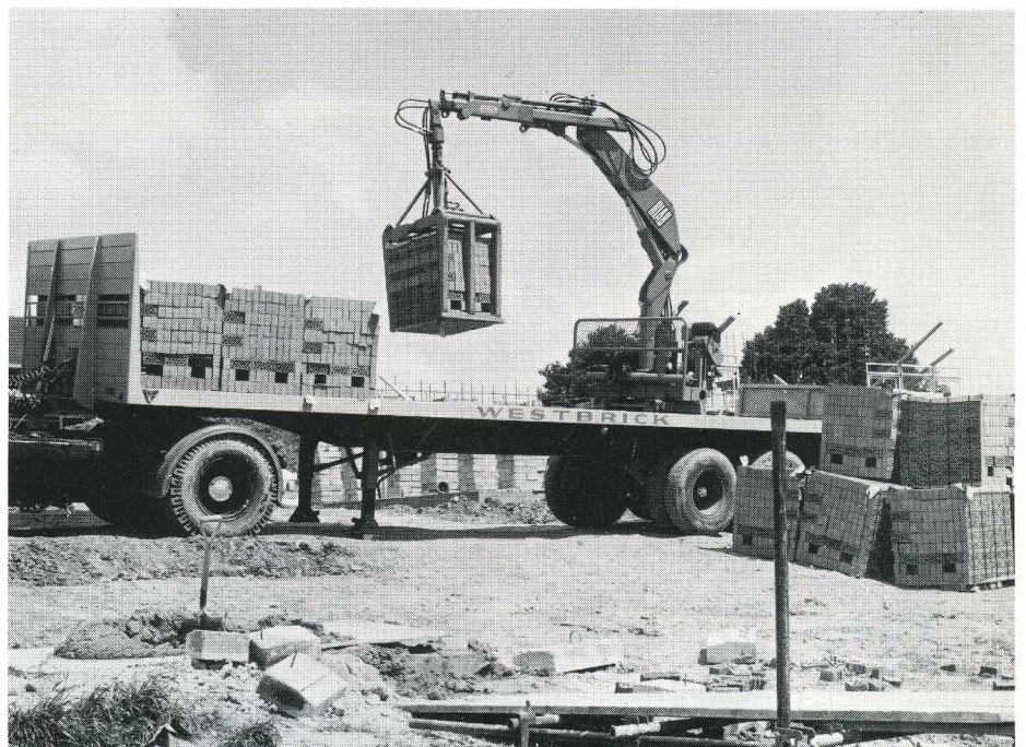
With a Rol-Loader-mounted HIAB 550, Frank Tucker can off-load 7,200 of Westbrick's facing bricks in 20 minutes. Using the time saved, he can get in another two delivery runs a day.
