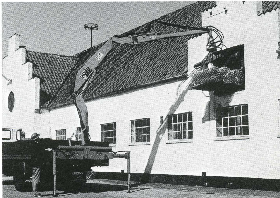
For greater stability under heavy lifts at large radius the support legs can be drawn out to a distance of 3.25 metres between the support points. In this picture only the right-hand leg is extended.
