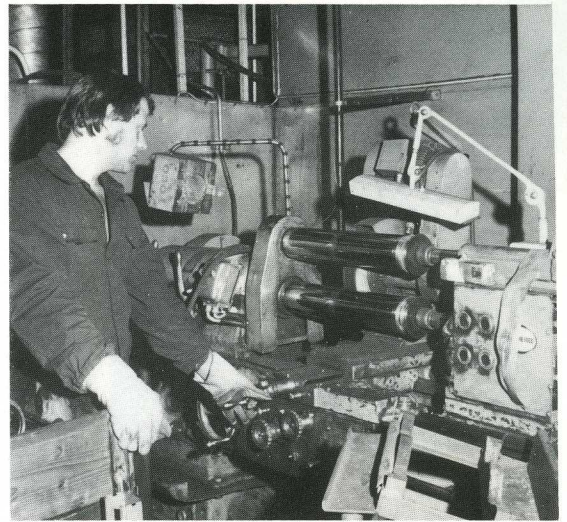
The polishing of the chromium plating is an important part of the surface treatment.
