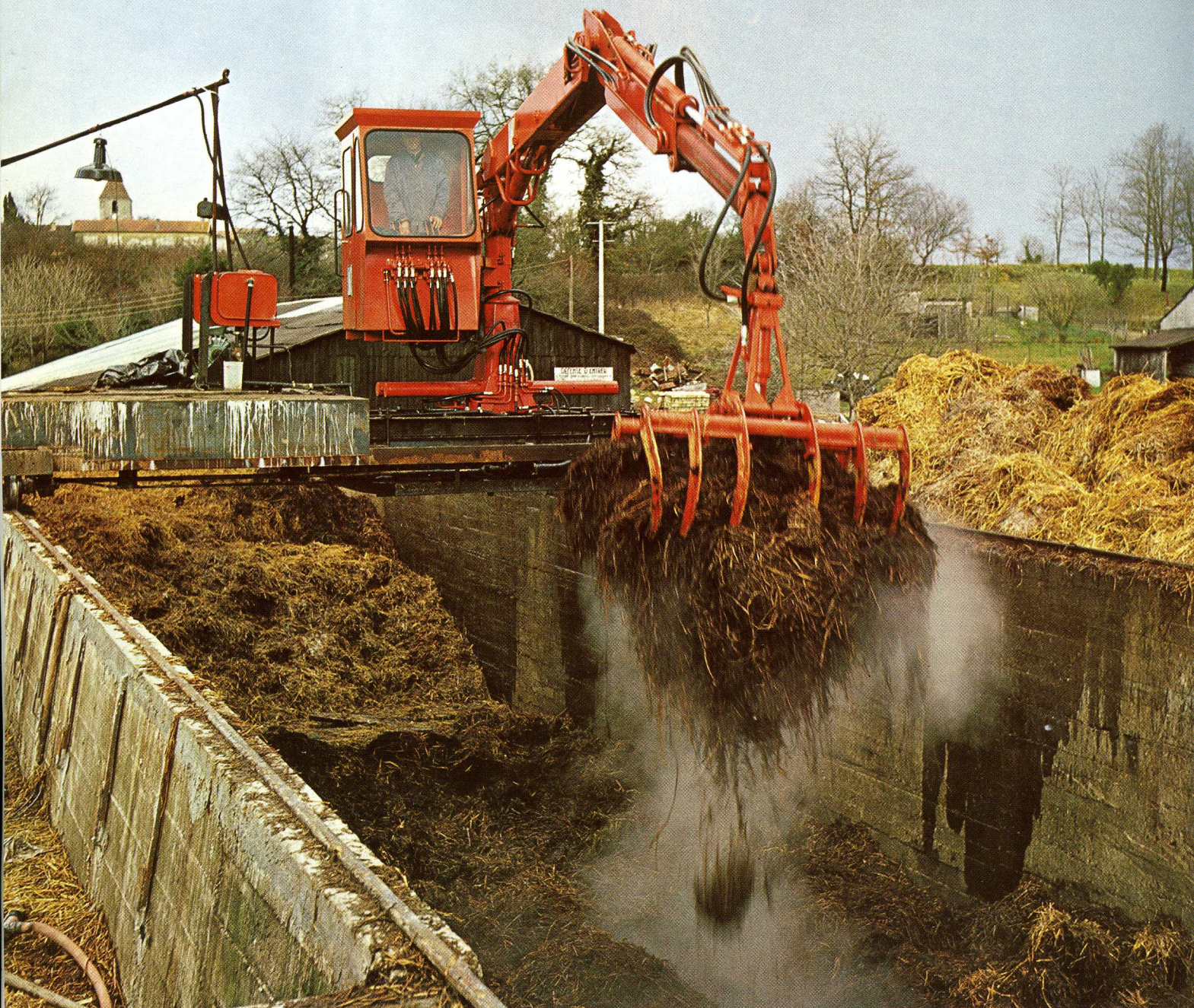
The compost mixture in the trench is ceaselessly worked over to achieve uniform consistency and to hasten decomposition. The loader is mounted on a gantry which can travel along the trench.
