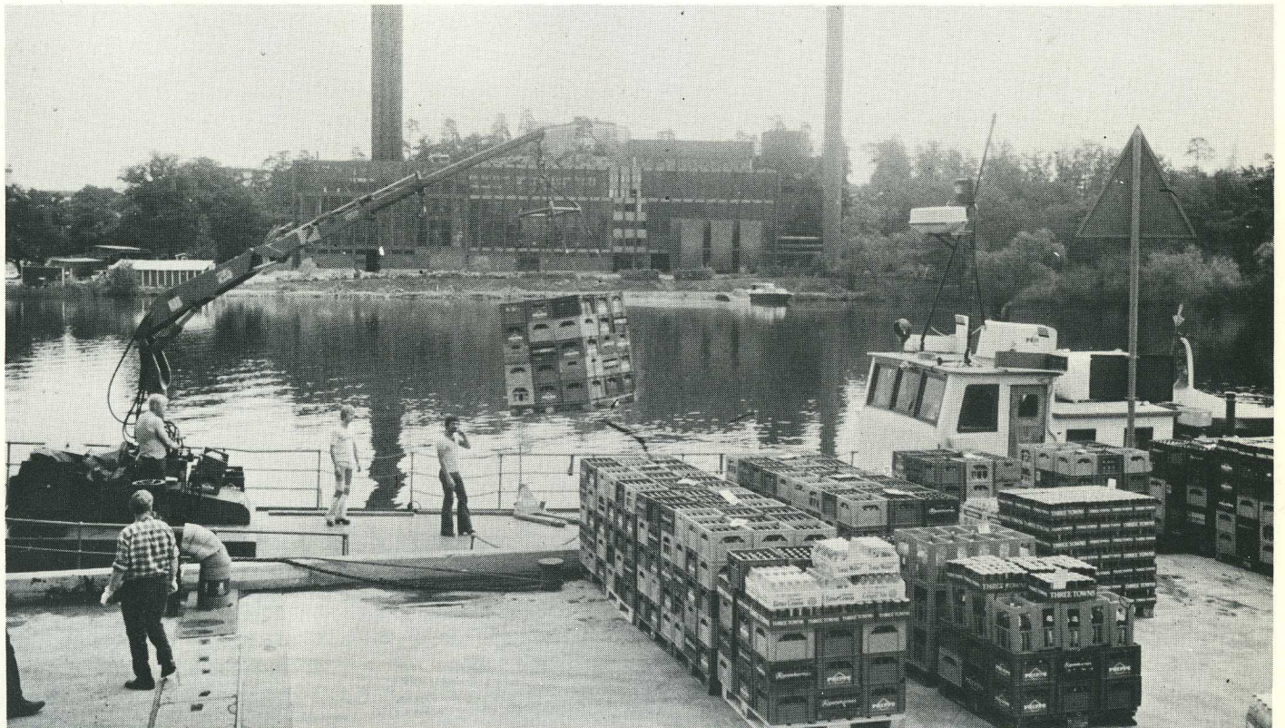
Time to load the deck cargo. The first pallet is already airborne, about 800 kg at full stretch of the boom. Thirty-odd must be loaded before the "Gambrinus" can cast off.
