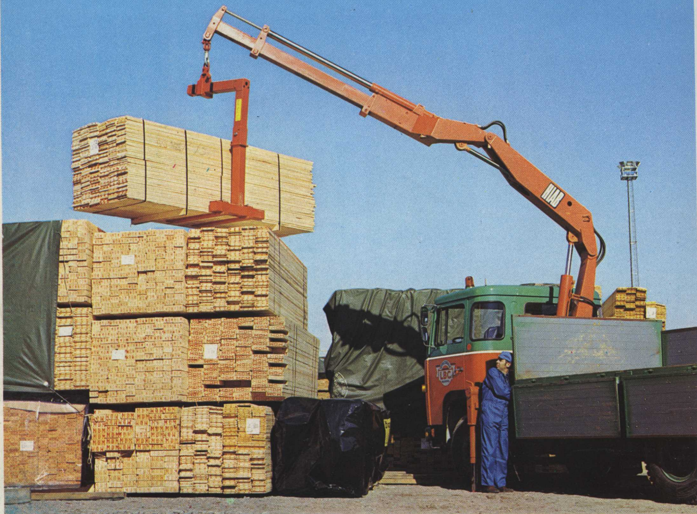
The HIAB 765 is a powerful loader. With its lifting moment of 7 ton-metres it can hoist weighty loads even on a long boom and to a great height.
