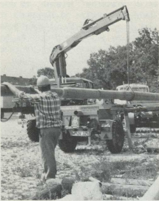
The lightweight outfit can also handle the loading of the posts onto a trailer.
