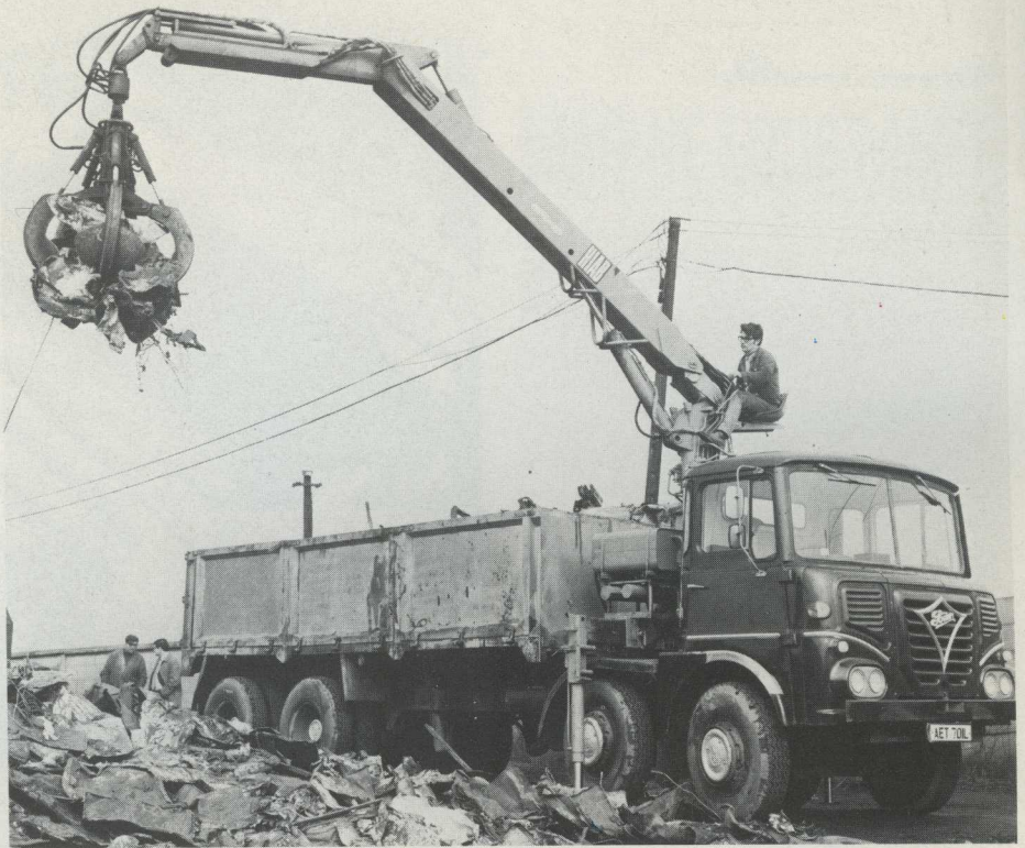
Thanks to its HIAB loader the lorry need never wait for the stationary crane at the collection site. Working alone, the driver loads up 16 tons in less than 30 minutes.
