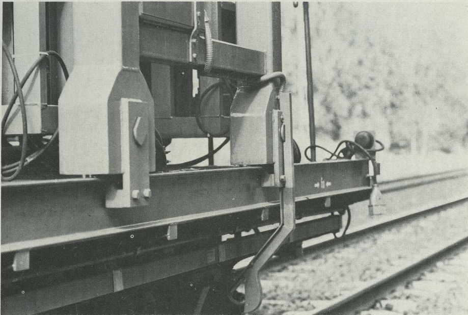
The loader, which has a much shorter body than standard, is mounted on a stout base which in its turn is arranged to travel the full length of the car. With this set-up the loader can put the cable drums straight into place in their cradles and then reach over them while the wire is being paid out.
