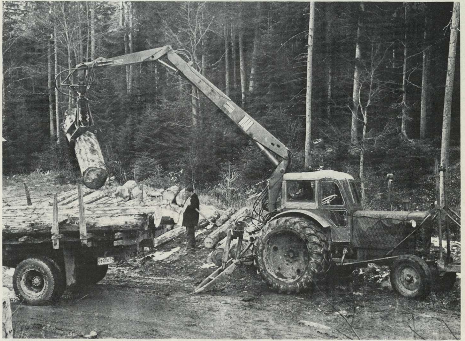
Large-sized timber is common in the Bulgarian forests, but the HIAB 560 has the necessary lifting moment. Sturdy support legs lend good stability to the tractor used as a mobile loader.
