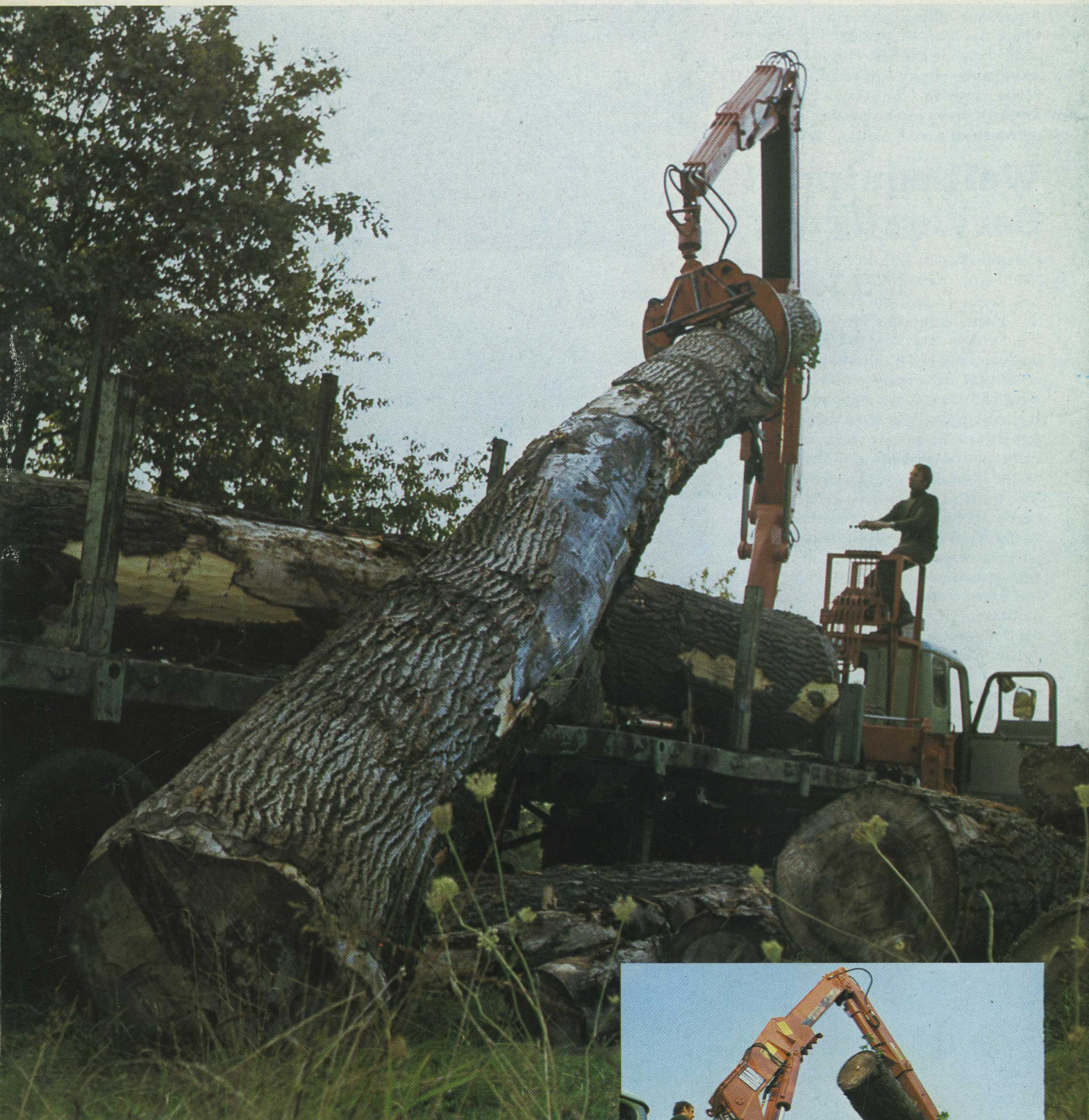
They're real hefty logs – but there's a real hefty loader to handle them, too. The HIAB 1560 wasn't designed as a forestry loader but its 15-ton-metre lifting moment comes in very handy on this particular job. The massive trunks grew in a French forest, where this outfit works.
