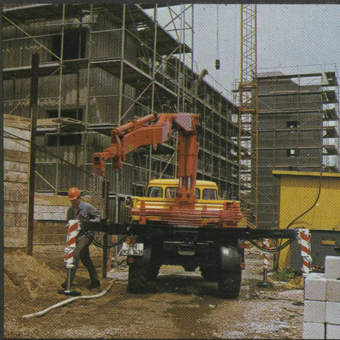
Four long extensible support legs give the lightweight truck the stability for heavy lifts.
