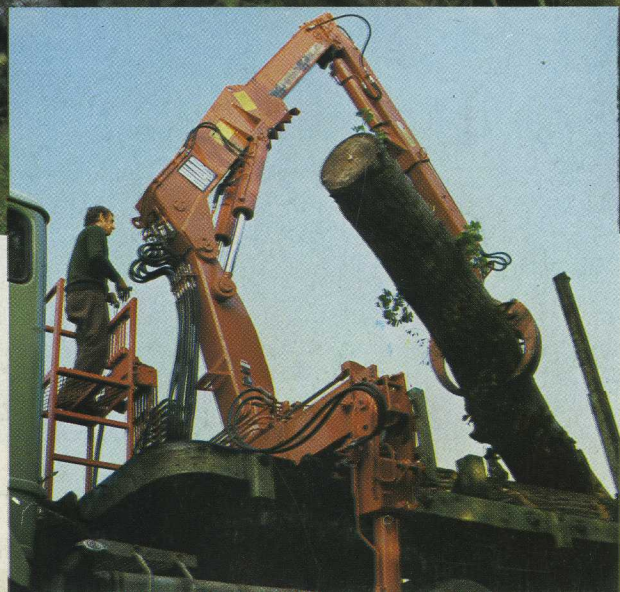
They're real hefty logs – but there's a real hefty loader to handle them, too. The HIAB 1560 wasn't designed as a forestry loader but its 15-ton-metre lifting moment comes in very handy on this particular job. The massive trunks grew in a French forest, where this outfit works.
