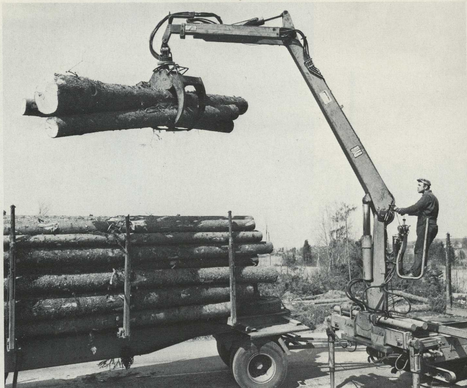
The brand-newest equipment for the grapple loading of roundwood: the HIAB 670 with the new, low-headroom, grapple, rear-mounted and platform-controlled.
