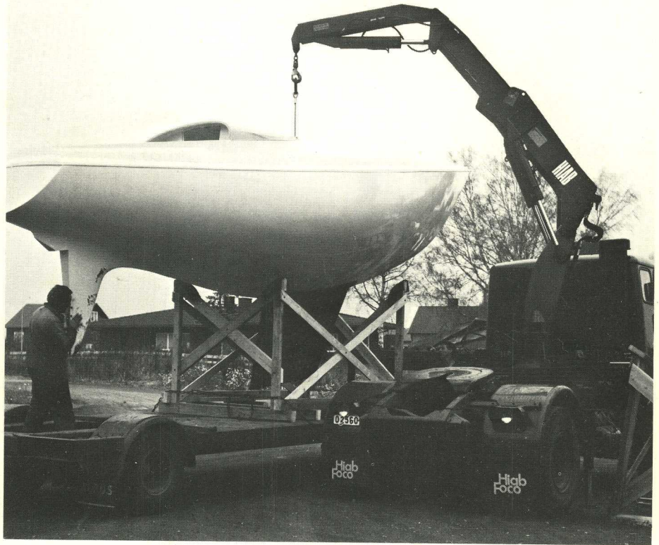
The great reach is a real boon when a sailing boat is to be lifted. The hook on this HIAB 1560 is a good five metres above the ground.
