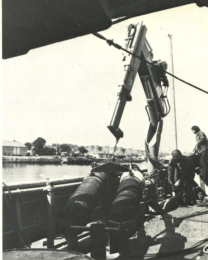
After lifting the guns from their cradles on board the loaders are able, thanks to their hydraulic extensions, to lower them right to the water surface without any hazardous swinging.
