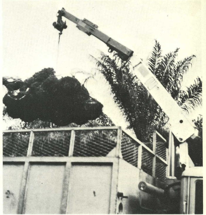
...but the net is emptied by an electromagnetic mechanism in the hook which releases three of the corners.
