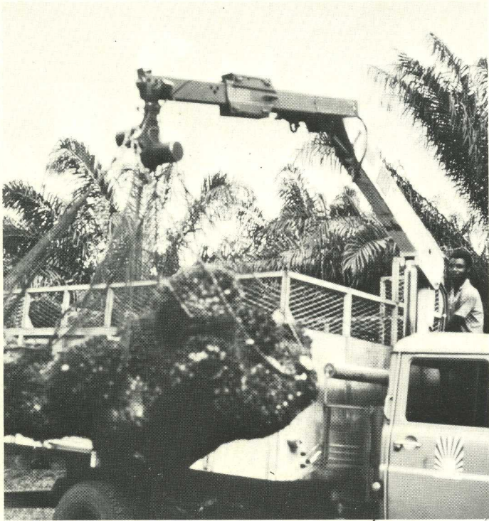
On the Palmivoire plantations, just as on the Nam Heng Estate, the oil-fruit is collected in a net that is hoisted by a HIAB 245...
