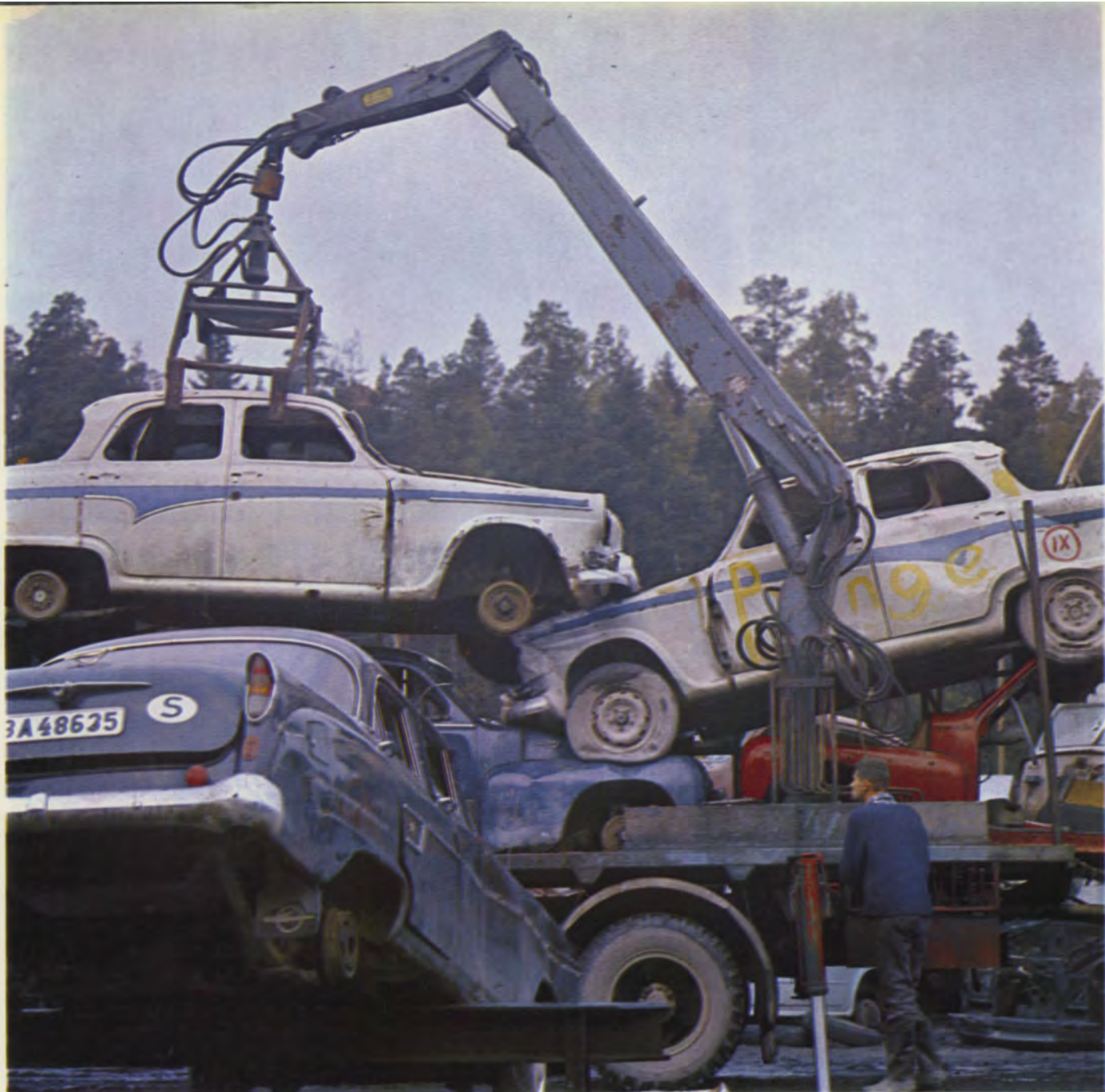
With a HIAB Speedloader and a special grab made for car bodies, Dan Liss can manage on his own the loading and unloading of the wrecks he moves to Gladö Kvarn. They're plentiful at this time of the year.
