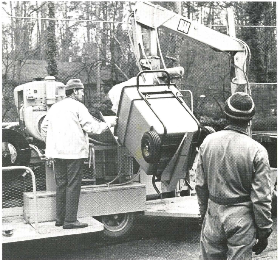
Collection is usually the most costly stage in dealing with refuse. Winston Salem has tackled the rising costs by mechanisation. The refuse bins are collected by a rubber-tired cart, and both the cart and the bin are lifted hydraulically for emptying.
