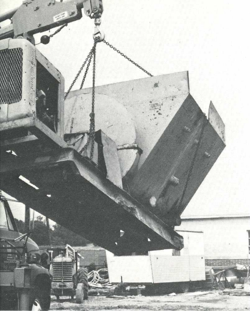
The heaviest stairways which Lennart Arvidsson handles weigh three tons, but the Hiab 950 can take the weight and outrigger legs give it the stability needed for spotting the stairway exactly in position.
