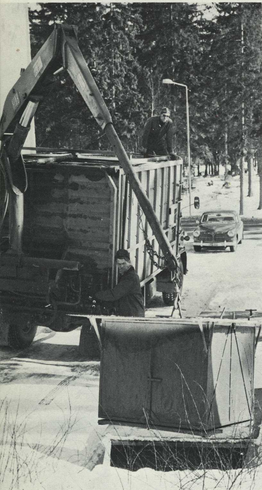
Using the Hiab Method the service company in Hagalund can handle the refuse containers with no trouble, even though the many architects who've made their mark on the area have each solved the problem of refuse storage in their own particular way.
