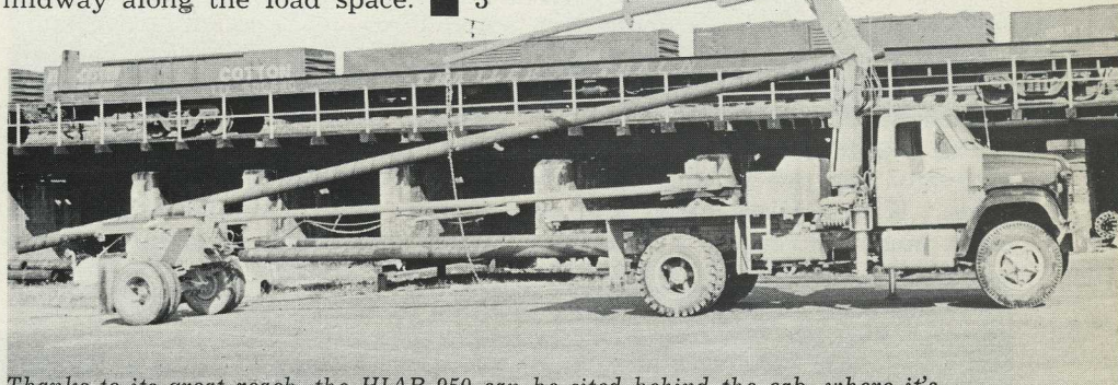
Thanks to its great reach, the HIAB 950 can be sited behind the cab, where it's out of the way, and can still lift the long pipes by their C. G.
