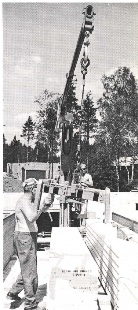
The B. Andersson trucking outfit is testing the HIAB 9501 on hauls of lightweight concrete. The loader is rear-mounted on a 33-foot semitrailer (left), and is used to unload both the semitrailer and a 30-foot trailer. Its hefty lifting moment and its long reach are valuable advantages in this kind of work.
