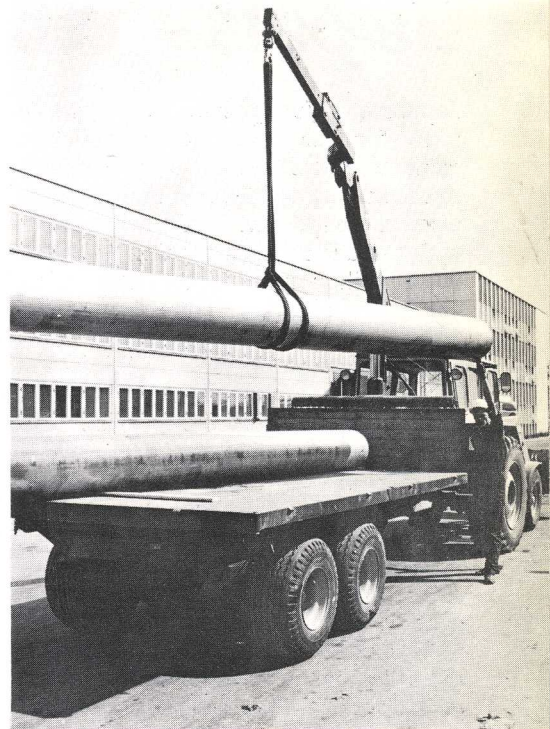
By having the loader mounted on the trailer it can be used in combination with any of the mill's tractors.
