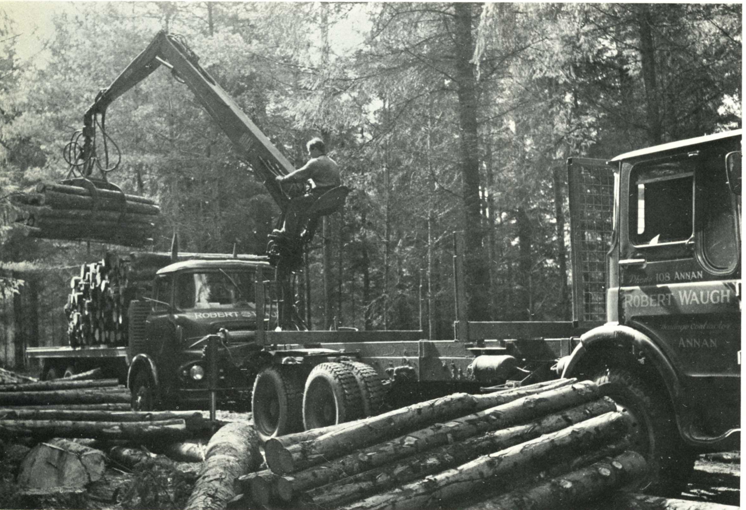
One further picture of the system adopted by Robert Waugh, the Annan firm of haulage contractors. Two vehicles—one with a HIAB 177—are normally sent into the forests, the HIAB loading both trucks with either mill timber or pulpwood, handling up to 26 tons of timber for the double load.
