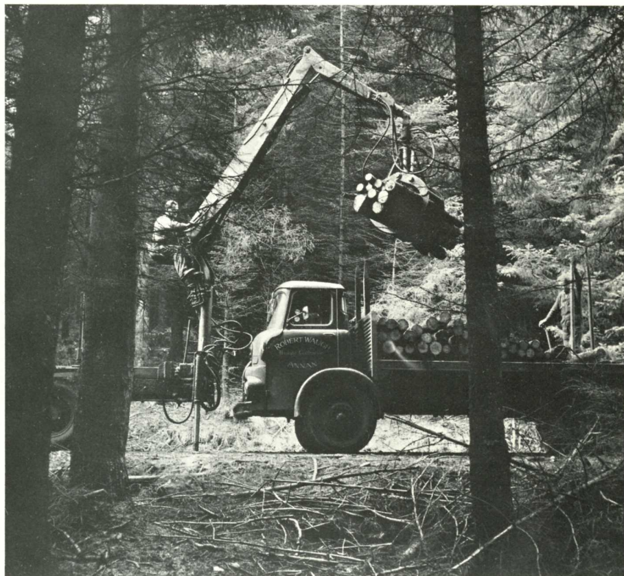
By letting two lorries operate as a pair, one of them equipped with a HIAB 177 which loads both vehicles, Robert Waugh of Annan, Dumfriesshire utilises the full capacity of the loader. Usually the pulpwood is loaded on the lorry without loader (pictures above and below) and the vehicle carries the mill timber. Loading is done in the afternoon and the 50 to 120 mile haul to Workington takes place in the morning.
