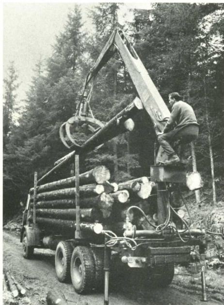
A HIAB 177, rear-mounted on a 6-wheel Dodge, picks up timber from dumps in the Kielder Forest. During the working day it collects four loads, each of around 12-13 tons, taking no more than 30 minutes to complete the pick-up.
