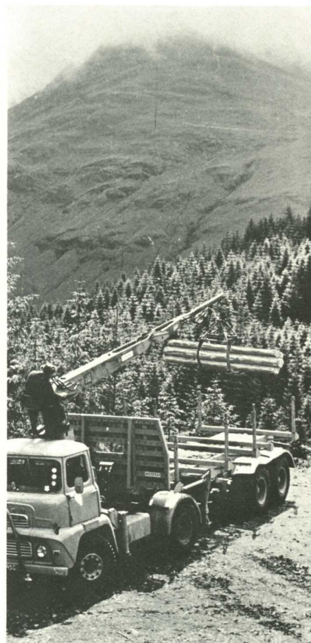
A HIAB 177, mounted behind the cab of a Dodge, at work in the forests around Inverinate, on the West coast of Scotland. This is one of the forests that serve the Wiggins Teape pulp and paper mill at Fort Williams supplying up to 1000 tons of pulpwood a day.
