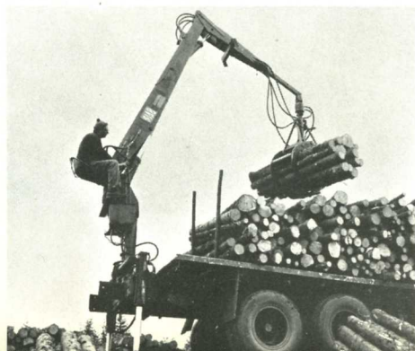
By letting two lorries operate as a pair, one of them equipped with a HIAB 177 which loads both vehicles, Robert Waugh of Annan, Dumfriesshire utilises the full capacity of the loader. Usually the pulpwood is loaded on the lorry without loader (pictures above and below) and the vehicle carries the mill timber. Loading is done in the afternoon and the 50 to 120 mile haul to Workington takes place in the morning.
