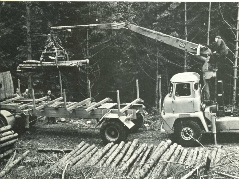
Flexibility is the keynote in any timber-handling system. Here at Inverinate, one Hiab loads two vehicles.
