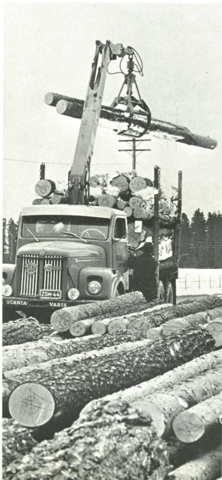
Grapple loading with the Hiab Method is rapidly gaining ground in Finland as the horses and the poorly equipped agricultural tractors in the forests are replaced by modern forest tractors. The low pile of timber that can be seen in the left picture below is the result of horse transport from the forest. With a forest tractor and the Hiab Method the logs can be stacked higher—more than two metres high—and the lorry can pick up a full load without having to change position during the loading.
