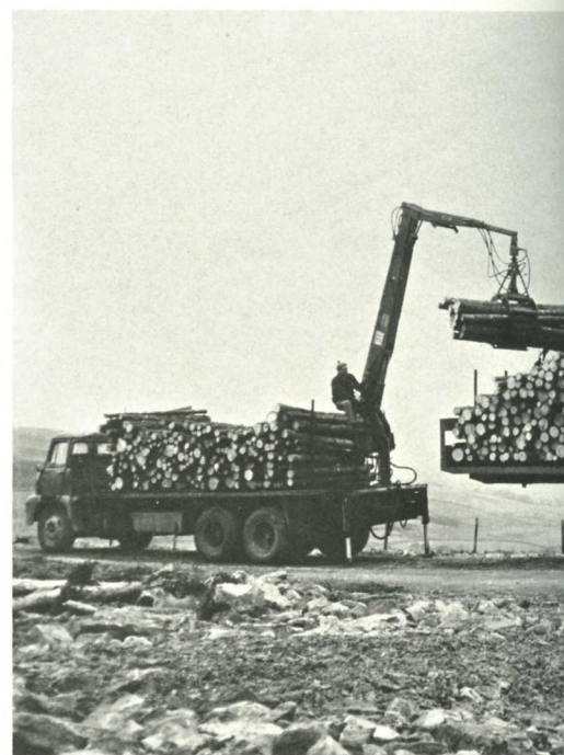
The next stage of the Kielder Forest load-delivery cycle. The Hiab off-loads the timber onto a waiting trailer, which is hauled by a Volvo tractor unit to the Workington board mill some 75 miles away.
