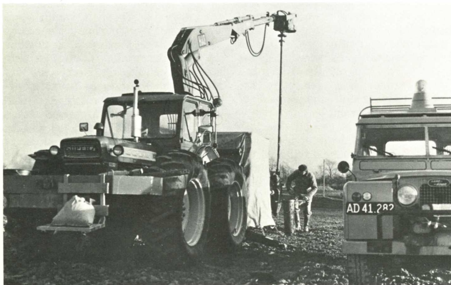
This earth drill equipment, frequently used by Danish electric power distributors, reduces the cost of making the hole for a pole or pylon to about 4 Swedish crowns compared to 24 Swedish crowns for a manually dug hole.
