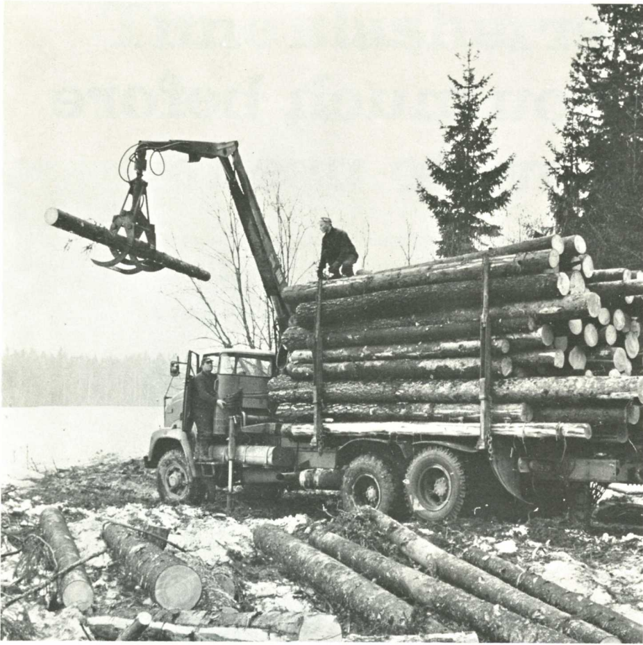
Grapple loading with the Hiab Method is rapidly gaining ground in Finland as the horses and the poorly equipped agricultural tractors in the forests are replaced by modern forest tractors. The low pile of timber that can be seen in the left picture below is the result of horse transport from the forest. With a forest tractor and the Hiab Method the logs can be stacked higher—more than two metres high—and the lorry can pick up a full load without having to change position during the loading.
