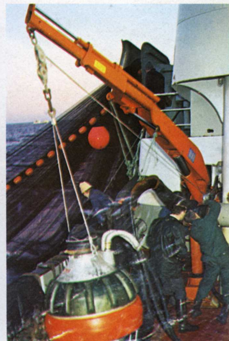
The ship's Hiab is used to manipulate the fish pump, and we saw for ourselves how smartly and effectively it carried out its important task during the hectic hours when the catch was coming aboard out on Haltenbanken.
