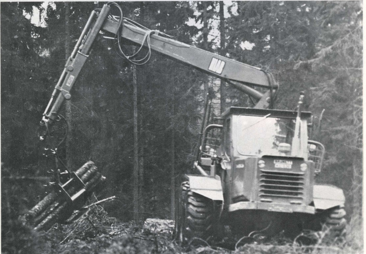
With a bogie on both the trailer and the tractor itself the new Brunett has an outstanding ability to keep going over bad ground and in deep snow.
