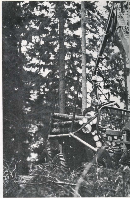
With a bogie on both the trailer and the tractor itself the new Brunett has an outstanding ability to keep going over bad ground and in deep snow.
