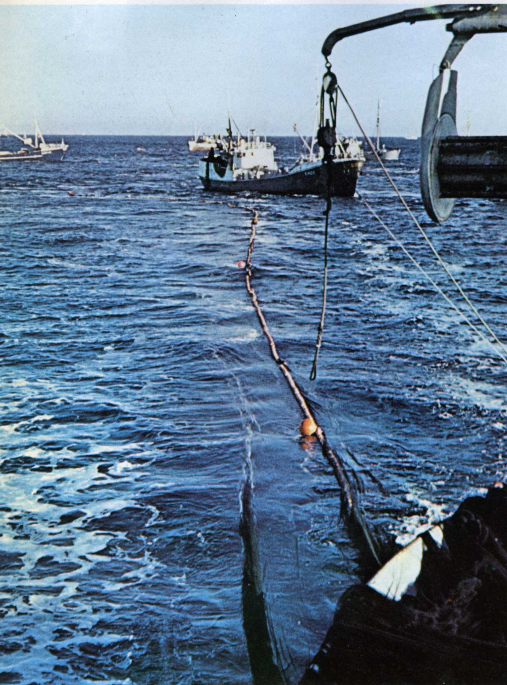
The ship's Hiab is used to manipulate the fish pump, and we saw for ourselves how smartly and effectively it carried out its important task during the hectic hours when the catch was coming aboard out on Haltenbanken.
