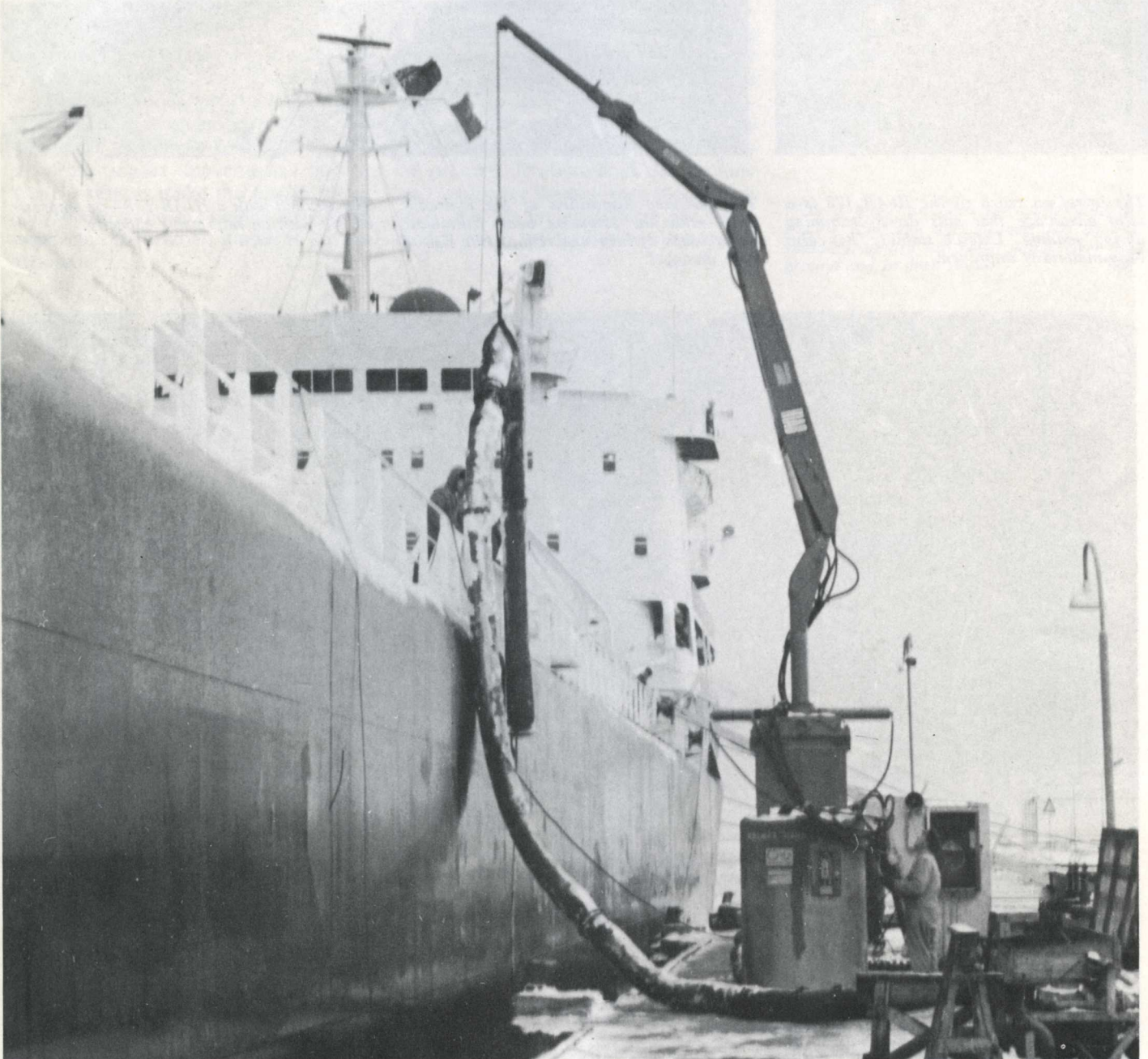
The rail of a lightly loaded 24,000-tonner is way above the wharf, but the long chain by which the hose is hanging shows that the HIAB 177 can manage the lift with plenty to spare.
