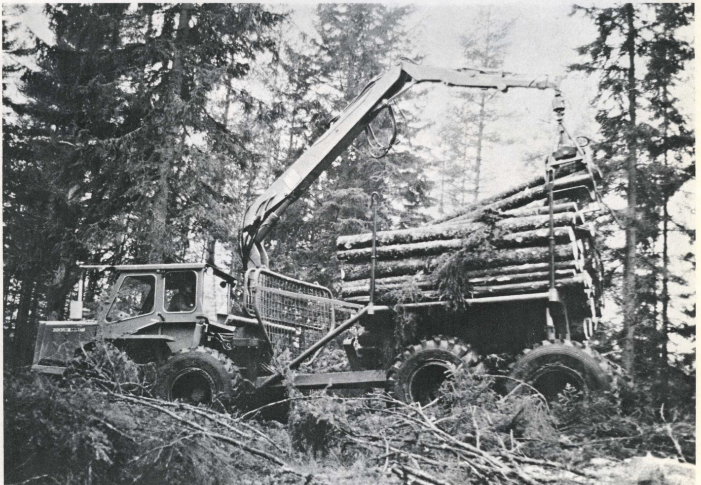
The increased reach of the HIAB 178 is a solid advantage that cuts down tramping during loading. Lateral stability has also been materially improved.
