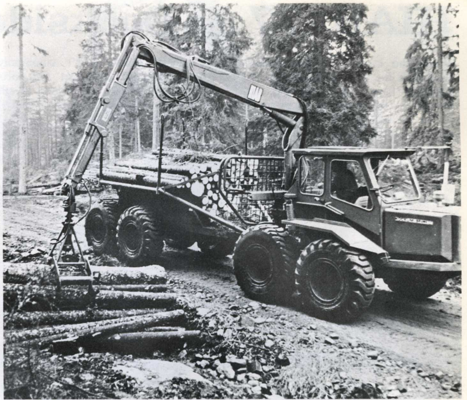
The sheltered disposition of the hydraulic lines inside the extension boom eliminates bulky loops of hose and reduces the risk of hose damage!
