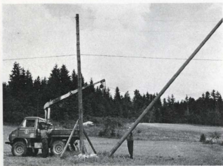
The limeworks at Lojo has a HIAB 293 equipped with a hydraulic winch.
