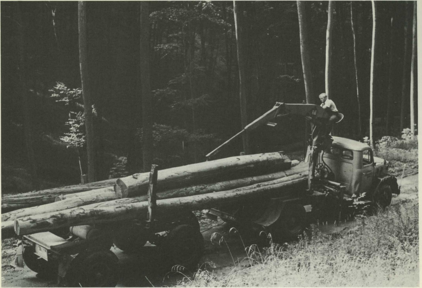
A trailer, a tractor truck mounting a HIAB 173 with a mast-top control seat behind the cab, an extra boom section, a log bar and a mechanical grapple—that's all the equipment German trucker Sielemann uses for moving long timber.
