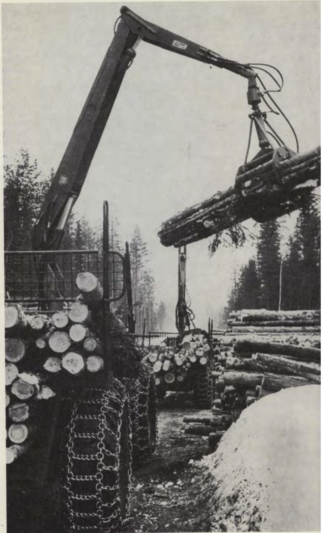
This picture shows unloading in progress down at the log landing by the motor road. The Speedloader enables the logs to be quickly stacked into piles over eight feet high, so that the landing can accommodate a great deal of timber on a relatively small area. Adjacent to the landing is a depot holding fuel for the tractors, etc.
